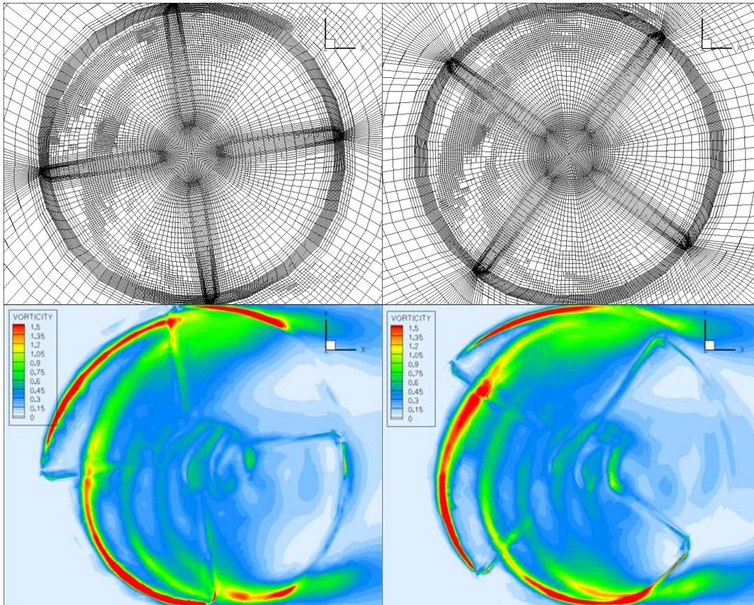
Figure 5 Locally refined meshes and flow results (vorticity magnitude) at azimuthal angle  $\Psi=9^\circ$  (left) and  $\Psi=54^\circ$  (right). Cross-sections are taken at  $z/R=0.085$ , where  $R$  is the rotor diameter and the hub center is located at  $z=0$ . Flow is from left to right.
