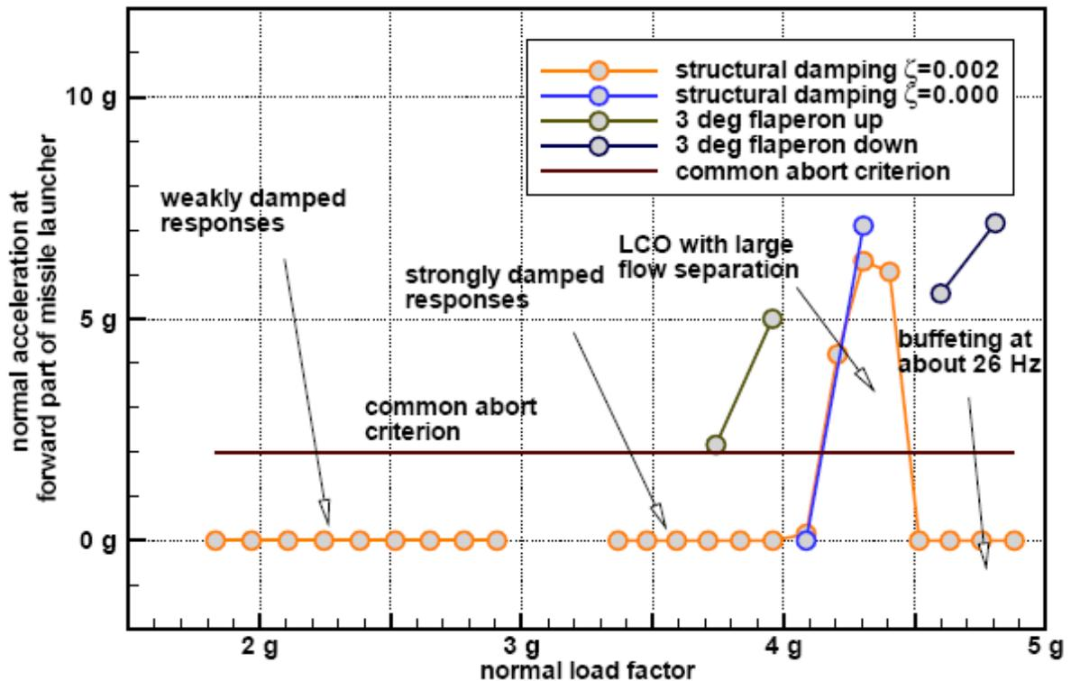
Figure 3 Diagram of LCO amplitude with respect to normal load factor for the F-16 aircraft;  $M_\infty = 0.90$ , FL100, Reynolds-Averaged Navier-Stokes flow model
