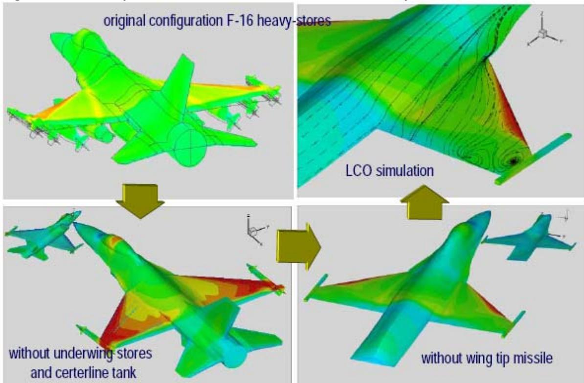
Figure 2 Reduction of the geometrical complexity of the F-16 heavy store configuration for the LCO simulation
