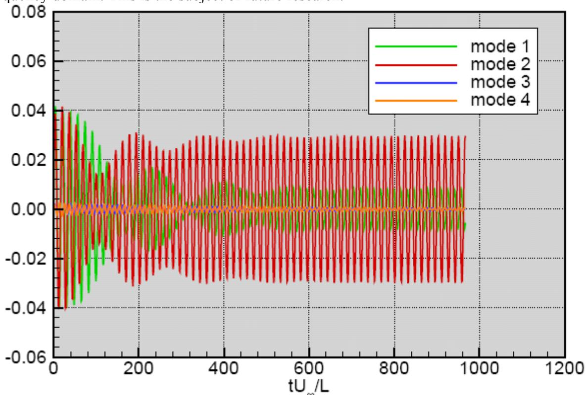
Figure 4 Time history of the generalised coordinates for the anti-symmetrical modes of the F-16 aircraft during the LCO simulation representing the dynamic deformation components;  $M_{\infty} = 0.90$ ,  $\alpha = 7$  degree, FL100, Reynolds-Averaged Navier-Stokes flow model
