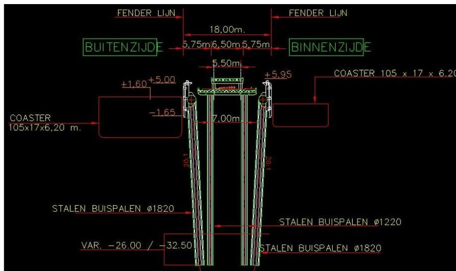
**Figure 2: cross section of the Lyondell jetty**
