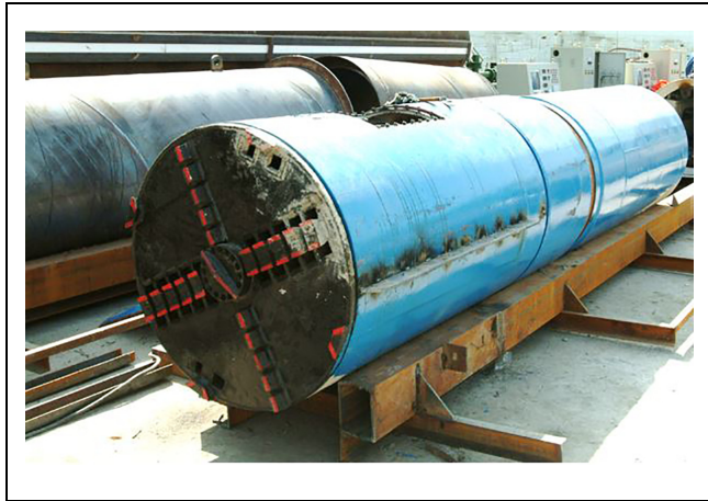
Figure 16. Slurry-type pipe jacking machine used in pipe umbrella installation.
