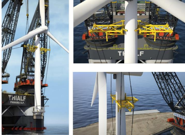
Figure A.8: Conceptual design of lift-frame for single-lift installation of WTG
