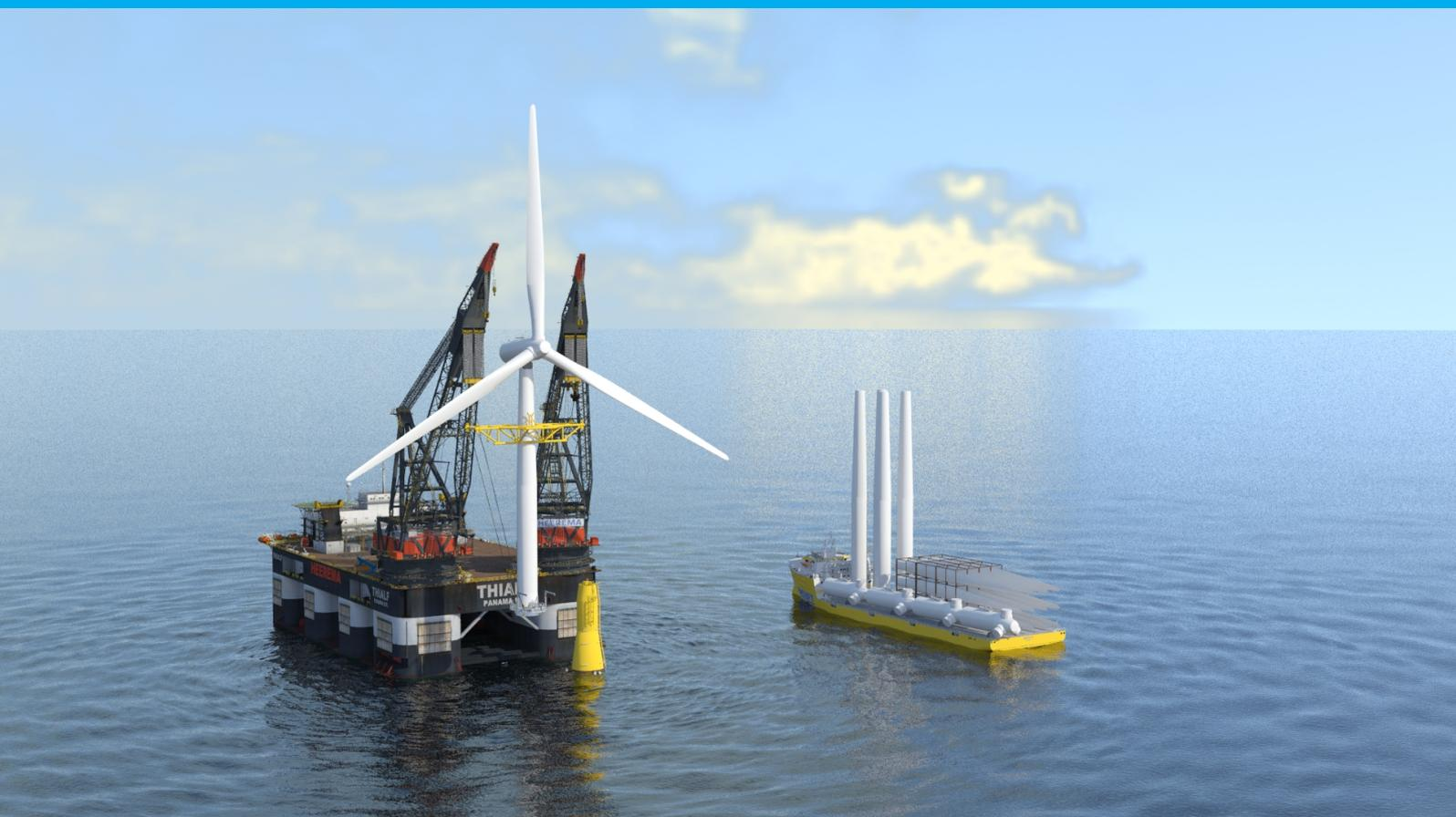
“Front cover: Graphical representation of a single-lift installation with the Thialf, where the wind turbine components are supplied per barge.”
