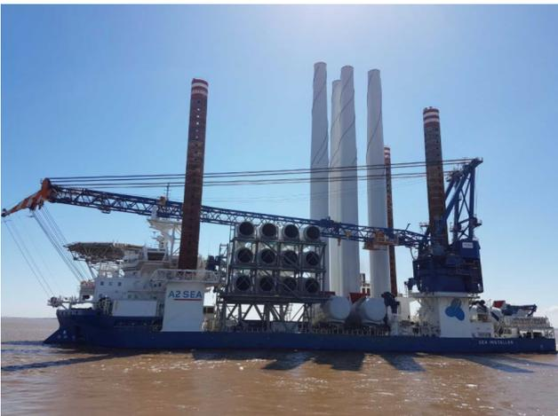
Figure A.1: 5 Pieces Separately with Tower in 1 Piece, SealInstaller – SeaJacks
