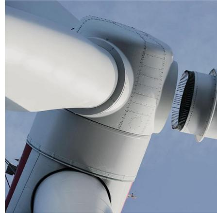
(b) Connection blade to rotor
