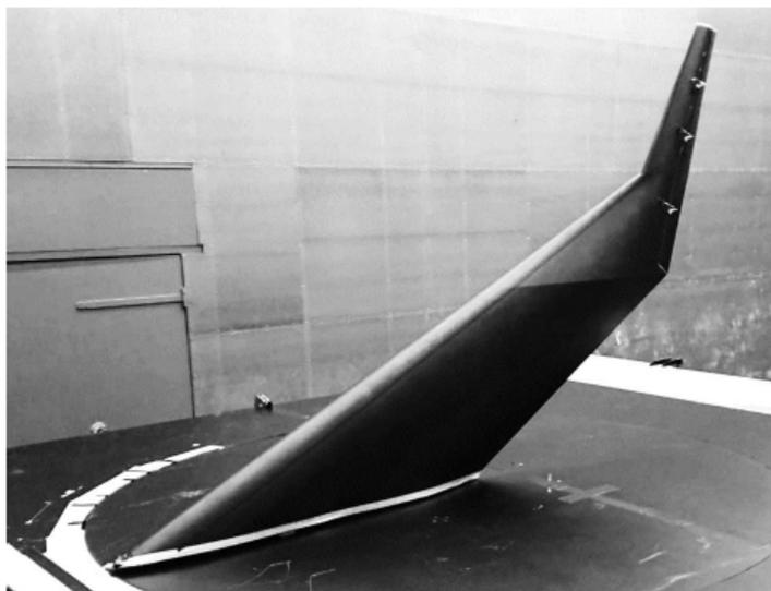
**Figure 2.3:** The original wind tunnel model constructed by Vos and Palermo [9]
