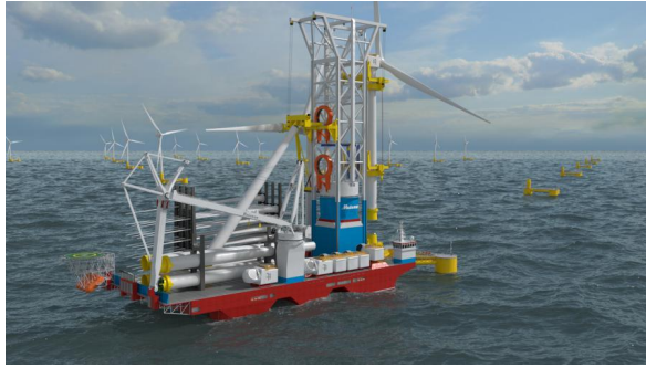
(a) The Huisman concept where the turbine is assembled offshore (Huisman Equipment)
