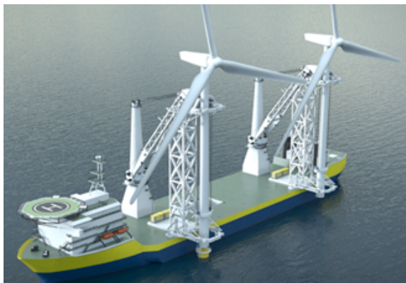
(c) The Offshoretronic installation vessel with their ADD-ON Installation Support Tower (Offshoretronic)
