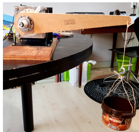
Figure K-2: Static Torque test Wheel-axle
