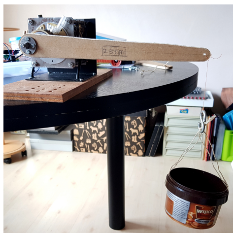
Figure K-1: Static Torque test Leg-axle
