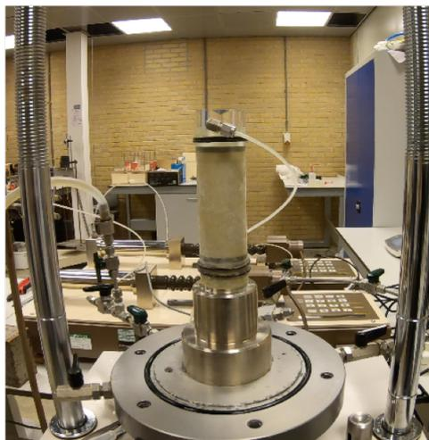
Figure 3.3: Triaxial test sample under vacuum
