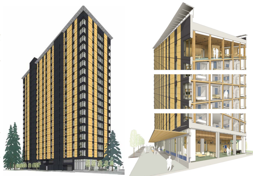
3D drawing of the building and perspective section. From bottom to top: Concrete structure with CLT canopy, encapsulated mass wood structure and exposed mass wood structure. (Source: Acton Ostry Architects)
