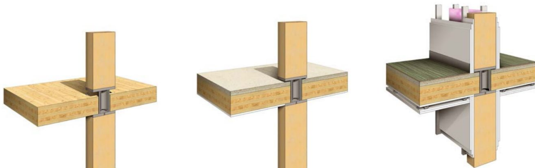
From left to right. 1. CLT floor slabs with glulam columns and steel connectors. 2. Partial encapsulation during construction. 3. Completed construction. (Source: Hermann Kaufmann)
