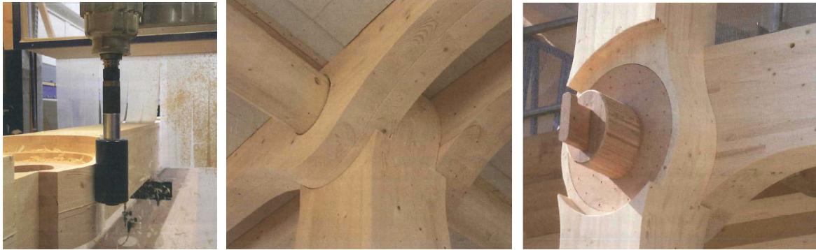
From left to right. Manufacturing of timber elements. Detail of column, beam, and ceiling interface. Detail of column and beam joint with hardwood connector dowel. (Source: Blumer Lehmann AG)
