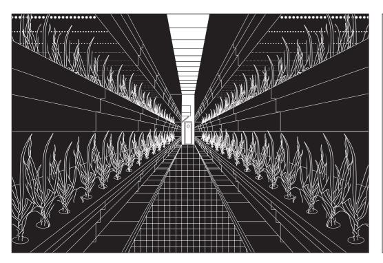
In controlled growth facilities a variety of rooms offer precise environmental control for the growth of high- or low-light plants, through the use of a top-down airflow pattern.
