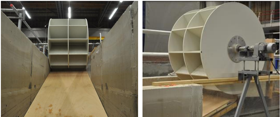
Figure 4 Front view and side view of the paddle wheel above the crest wall.
