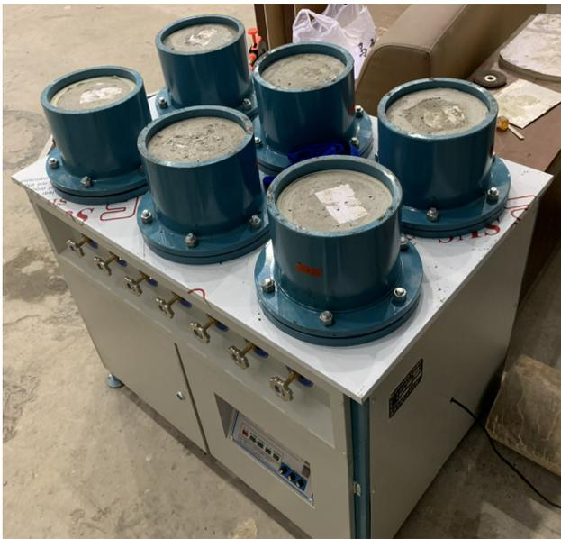
Fig. 11. Permeation test apparatus.
