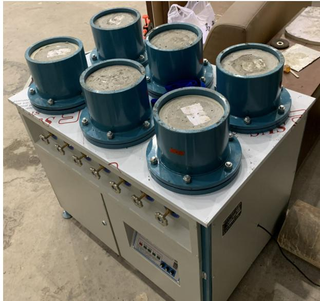
Fig. 11. Permeation test apparatus.
