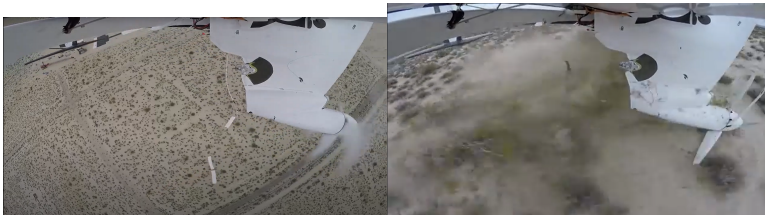
Figure B.2: Rupture of tether (left) causing a controlled crash (right) [148].
