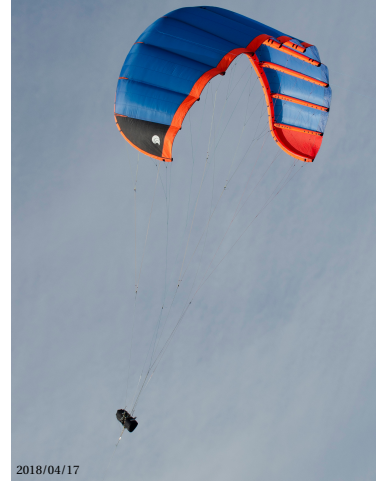
Figure 3.2: A, Front view of the leading-edge inflatable (LEI) V3 kite [60]; B, Photo of the V5.40 with 40 m 2 wing surface area (courtesy of Kitepower B.V.).
