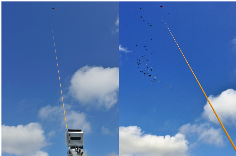
Figure B.8: Photo sequence capturing a bird impacting the tether: before the impact (left) and shortly after the impact (right). Photo: Max Dereta
