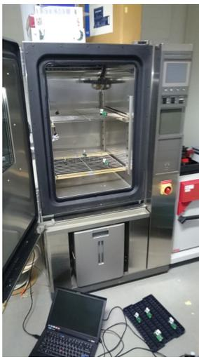
**Figure 8-2:** The climate chamber used for the temperature experiments. Some nodes are visible inside the chamber and on the ground in front of it.
