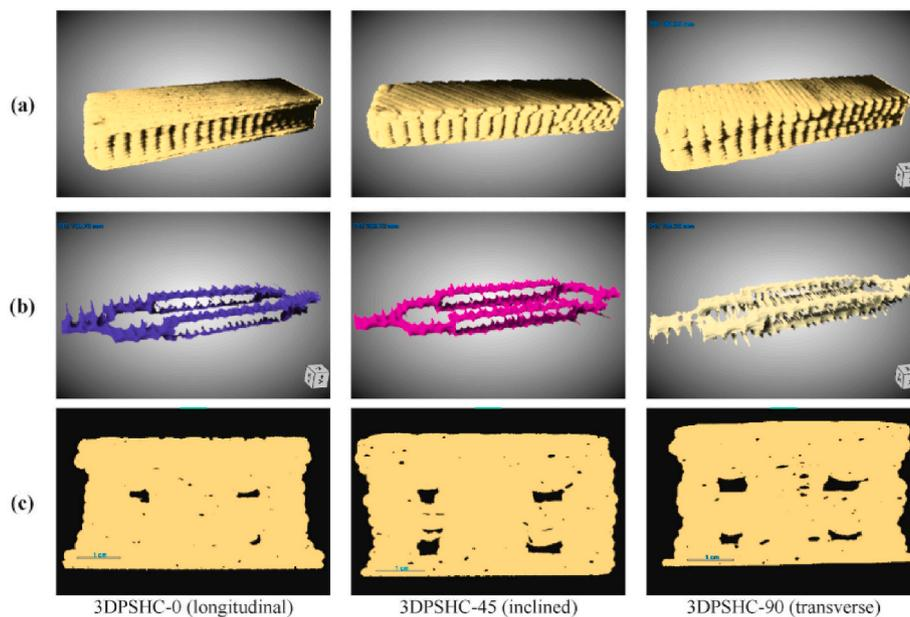
Fig. 18. Reconstructed CT results of 3D-printed vascular self-healing cementitious materials (Wan et al., 2023b).
