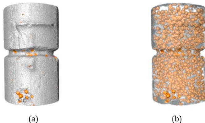
Fig. 2. Capsule based self-healing concretes (Lv et al., 2017) (a) Paste cylinder; (b) Microcapsules in cementitious matrix.
