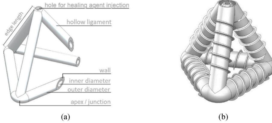
Fig. 12. (a) Schematics of a MVN unit (De Nardi et al., 2020); (b) d-TET housing two-component healing agents (De Nardi et al., 2023).
