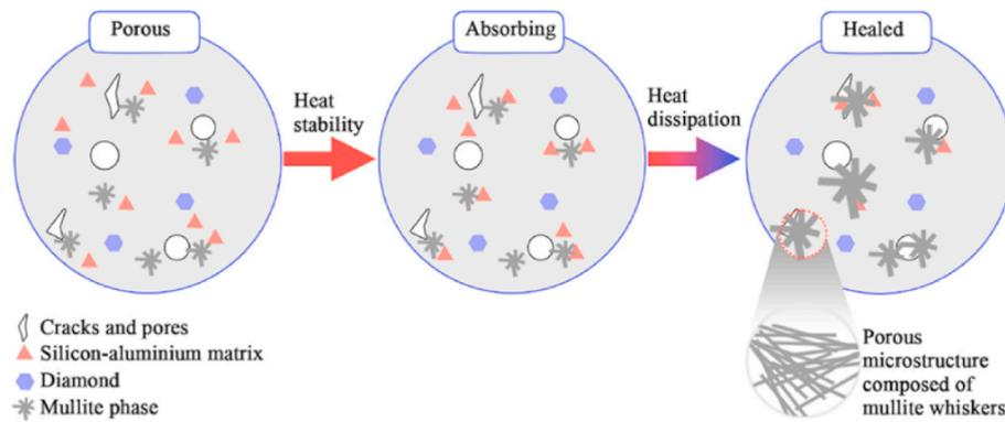
Fig. 16. Schematic of self-healing mechanism in DPG (Tang and Tang, 2022).
