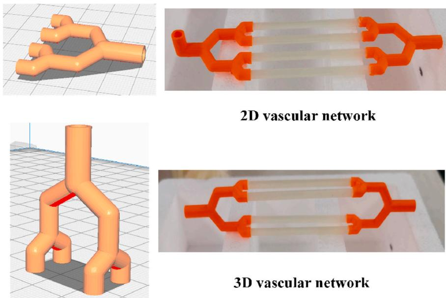
Fig. 11. Schematics of 3D-printed PVA vascular networks (Wan et al., 2023a).
