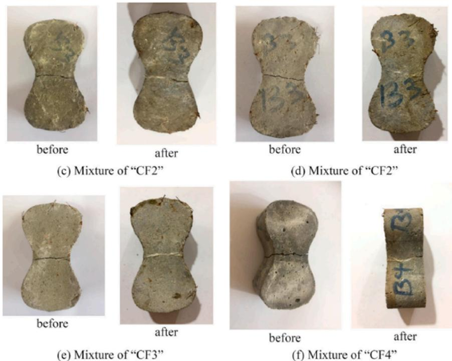
Fig. 14. Crack sealing of 3DCP with steel fibre coated with PVA and GO (graphene oxide) (Ahmadi et al., 2023).
