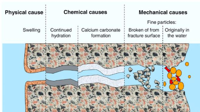
Fig. 1. Mechanisms of autogenous self-healing (Rooij et al., 2011).
