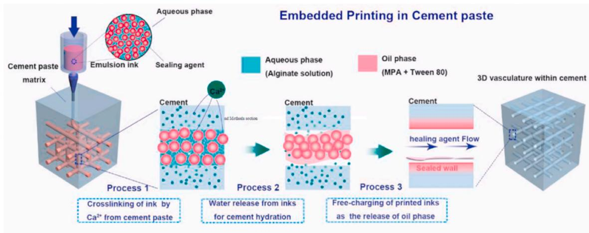
Fig. 17. Schematic of 3D printing of vasculature in cementitious matrix (Zhang et al., 2022).
