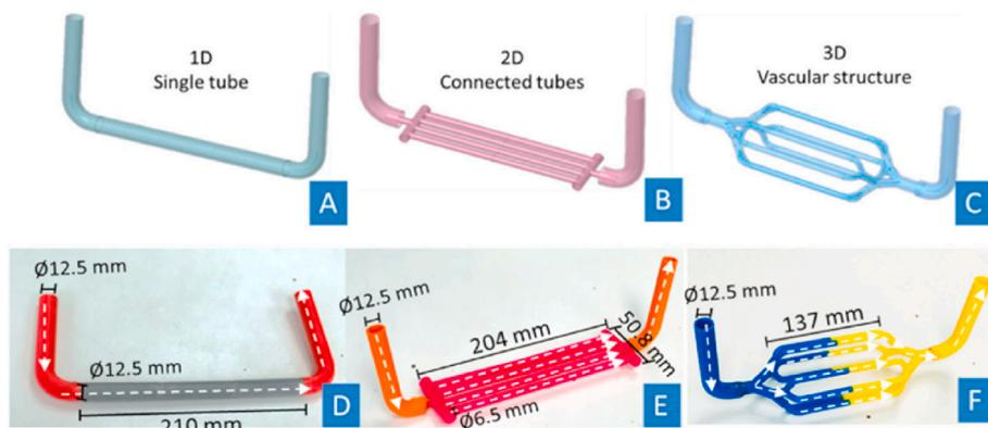
Fig. 9. Schematics of designed 1D/2D/3D vascular structures (Li et al., 2020).
