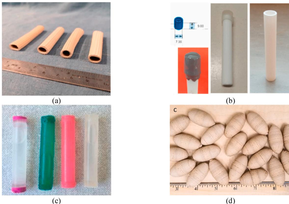
**Fig. 5.** (a) Extruded cementitious hollow tubes ([Anglani et al., 2020b](#)); (b) 3D-printed acrylate/ceramic capsules ([Riordan et al., 2023](#)); (c) 3D printed capsules (from left to right PMMA, PET, PLA, PETG) ([Anglani, 2019](#)); (d) Lignin-based capsules ([Sinha et al., 2022b](#)).
