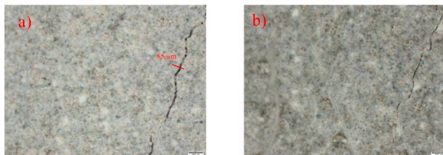
Fig. 15. Preloaded crack in the 3D-printed ECC in curing chamber. (a) 2 days; (b) 28 days (Fernández et al., 2023).
