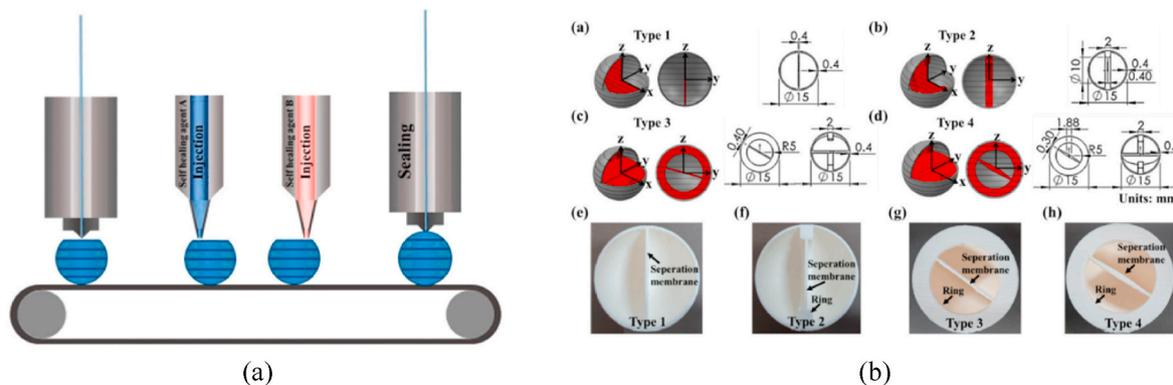
**Fig. 6.** Capsules that house two-component healing agent (a) fabrication of two-component capsules; (b) design of four types of capsules that house two-component healing agent ([Lim et al., 2023](#)).
