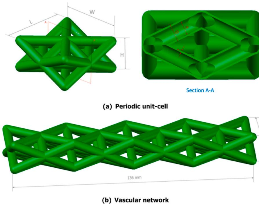
Fig. 10. Schematics of 3D-printed ABS vascular networks (Wan et al., 2022a).
