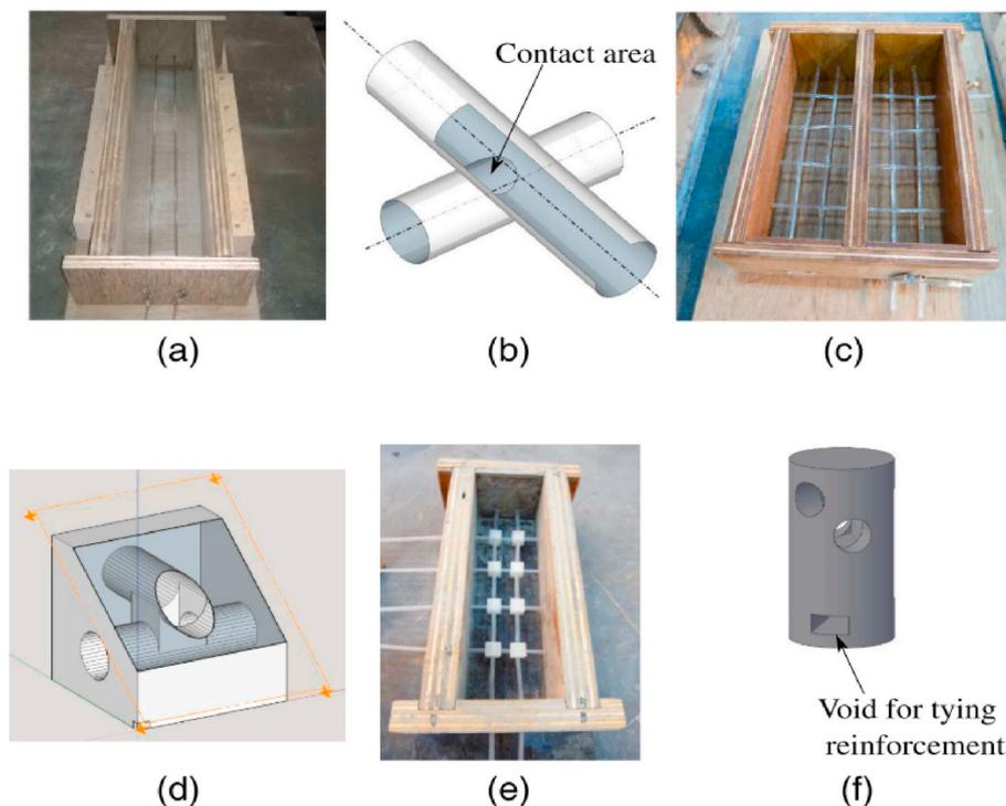
Fig. 7. 2D vascular system in the mould for casting (Davies et al., 2021).
