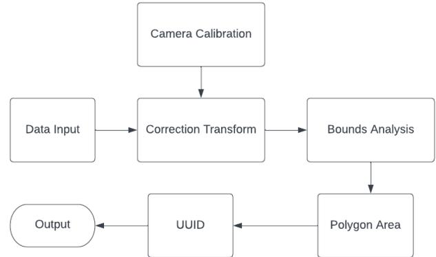
Figure 4: The pre-processing pipeline
