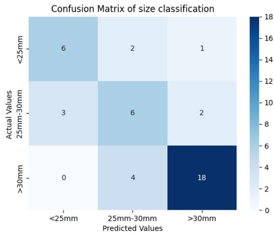
Figure 10: A confusion matrix showing the predicted and actual values of the size labeling using depth estimation
