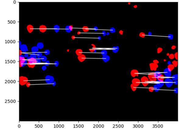
Figure 7: Potential Matches. Red segments are strawberries from the right camera. Blue segments are strawberries from the left camera. A white line indicates a potential match after variable constrains
