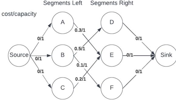
Figure 8: An example network model for matching the left and right segments
