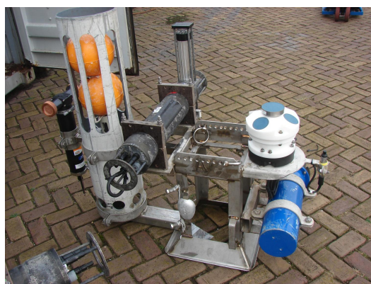
Figure 4.3: AWAC measuring system setup used in the outer harbor (source: RWS [37])
