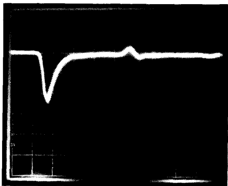
Fig.5: Output signal of the XP2020 PM, generated by heavily degraded 200 MeV/c antiprotons. Horizontal: 10 ns/div.; vertical: 0.5 V/div.
