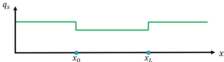
Figure 2.14: Sediment transport gradients resulting from a coarsening of a river reach.
