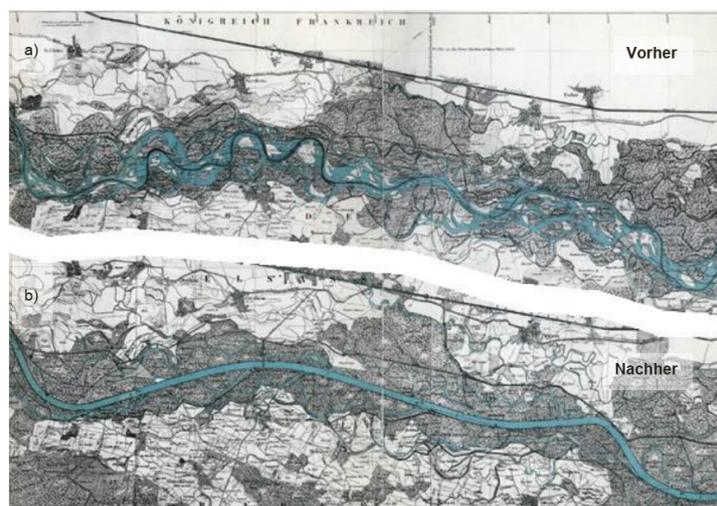
Figure 1.1: Rhine reach between Weisweil and Marlen. On top the meandering river reach before the normalisation works. On the bottom the same straightened river reach afterwards. (Hillebrand et al. 2017)
