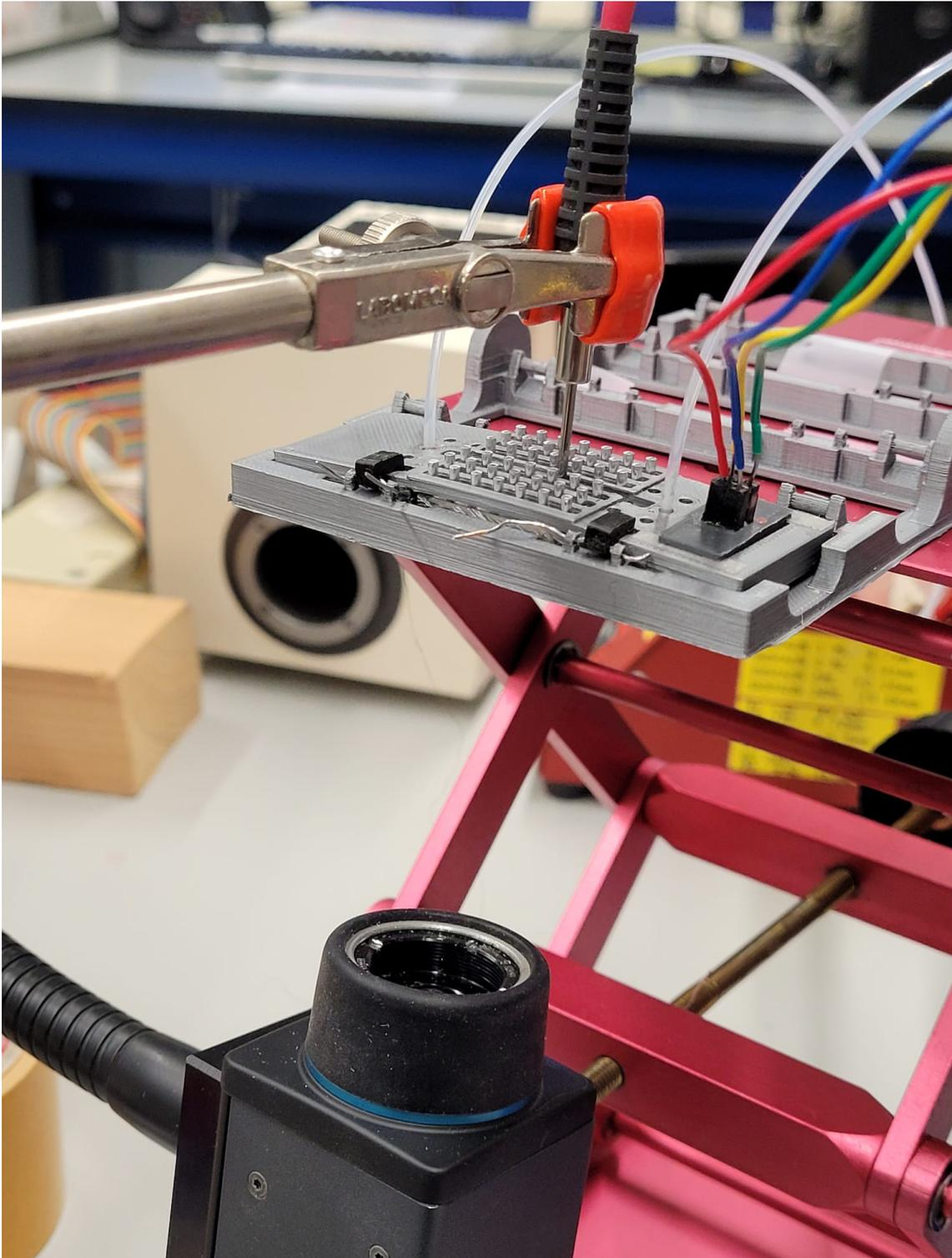
Figure A3: Test setup for Oxygen measurements close up
