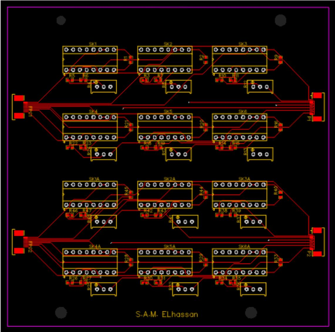
Figure C4: Layout PCB, top connections
