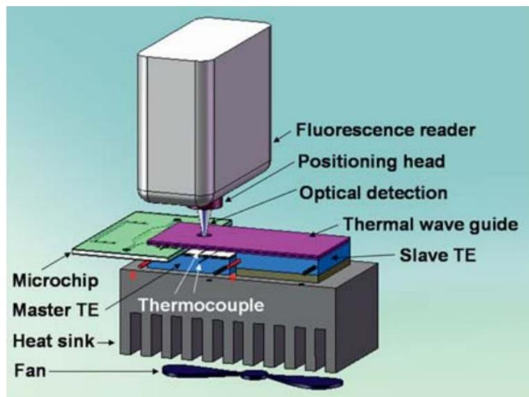
Figure 6: Schematic drawing of the real-time PCR platform with the microchip partly inserted [11]
