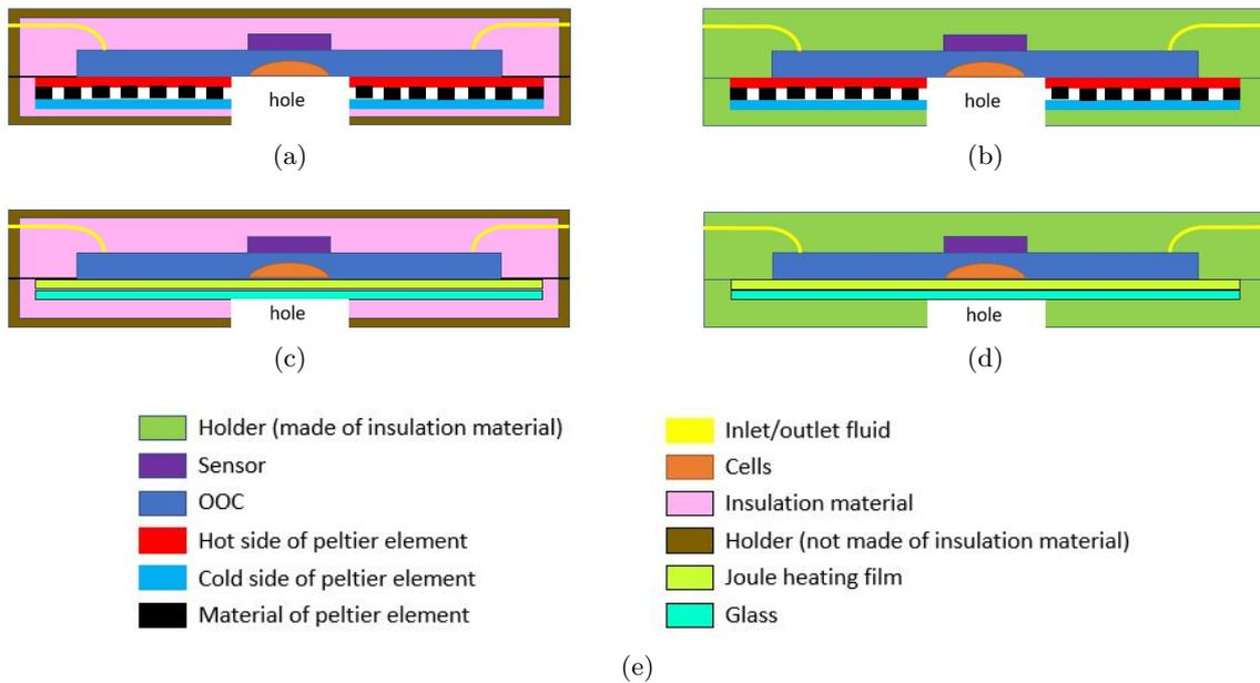
Figure 20: (a) Peltier design where the holder and insulation material are not the same (b) Peltier design where the holder and insulation material are the same (c) Thin film Joule heating design where the holder and insulation material are not the same (d) Thin film Joule heating design where the holder and insulation material are not the same (e) Legend
