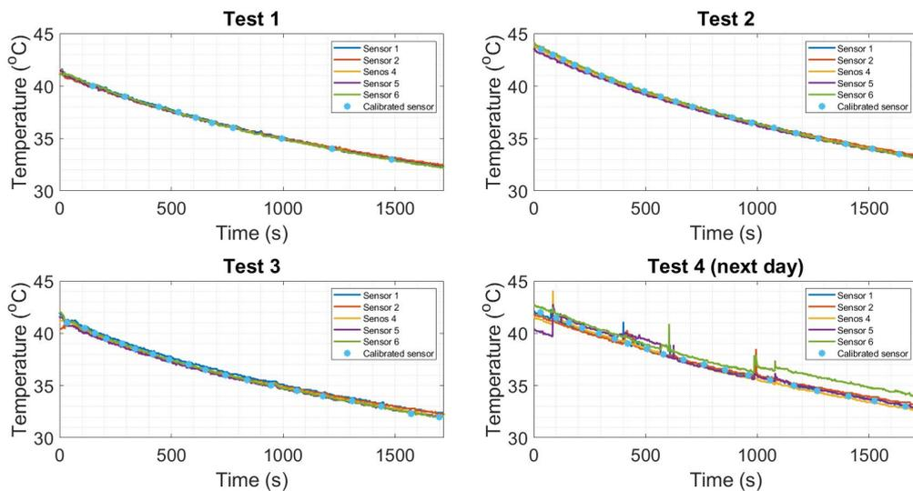
Figure G3: Four experiments with 5 RTD sensors and one calibrated sensor. The calibrated sensor is a thermometer (similar to Medisana, Medisana TM-700) used to measure the temperature of a human. The fourth experiment was done on the next day. This shows that the sensor values can change over time. This was most likely due to the fact that the cables were connected to a breadboard which was unstable, which changed the value of the resistance of the RTD sensors
