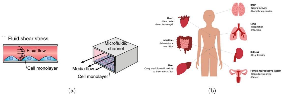
Figure 2: (a) Schematic of a OoC [1] (b) An overview of organs that can be used in OoC and the diseases that can be modelled [5]
