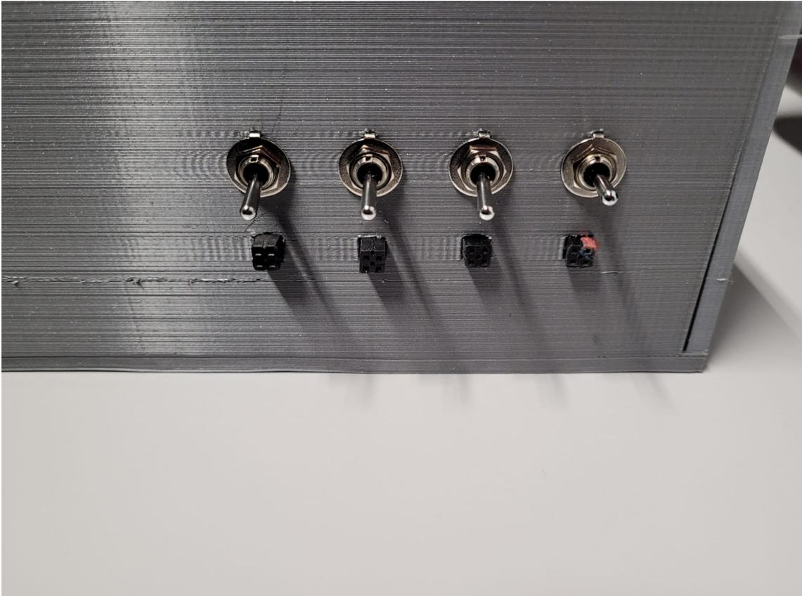
Figure E8: A close-up of the switches and cable connectors. Switching up is heating, down is cooling and in the de middle is off
