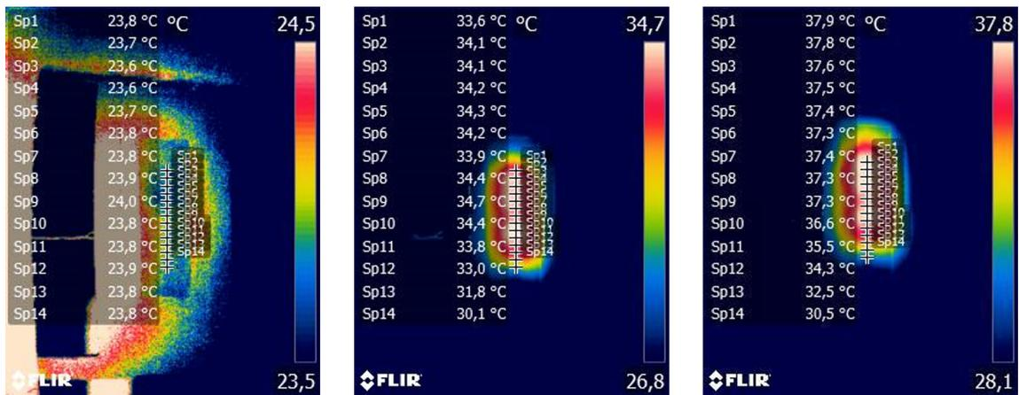
Figure G5: Thermal images of a test of heating from room temperature. Fluid flow was from sp14 to point sp1 and was  $35 \mu\text{L}/\text{min}$
