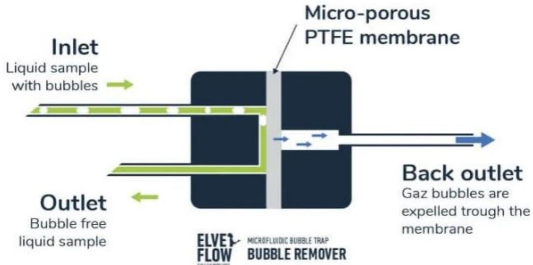
Figure 16: A schematic drawing of a bubble trap [22]
