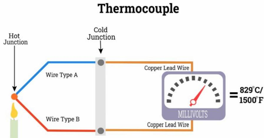
Figure 10: Principle of a thermocouple [16]
