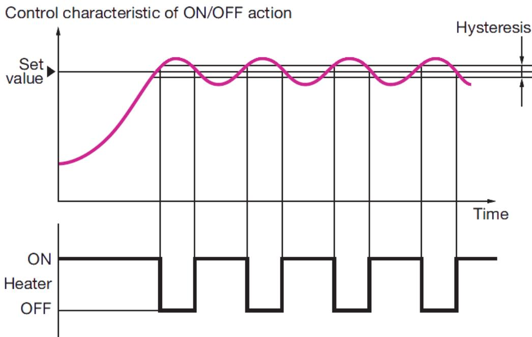
Figure 13: Graph of an On-Off controller [20]
