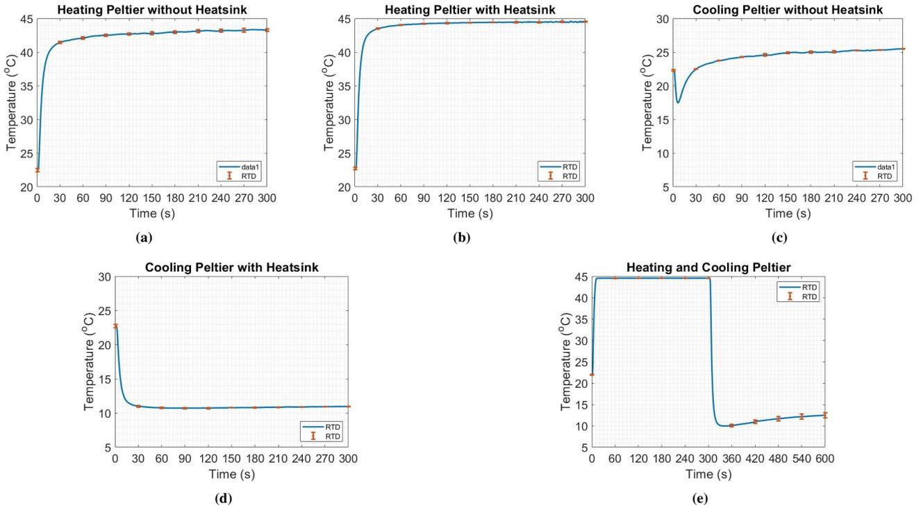
Fig. 8: For the schematic drawing of the experiments see Figure 5a (a) Peltier heating without heatsink for five minutes (b) Peltier heating with heatsink for five minutes (c) Peltier cooling without heatsink for five minutes (d) Peltier cooling with heatsink for five minutes (e) Peltier first 5 minutes of heating than 5 minutes cooling
