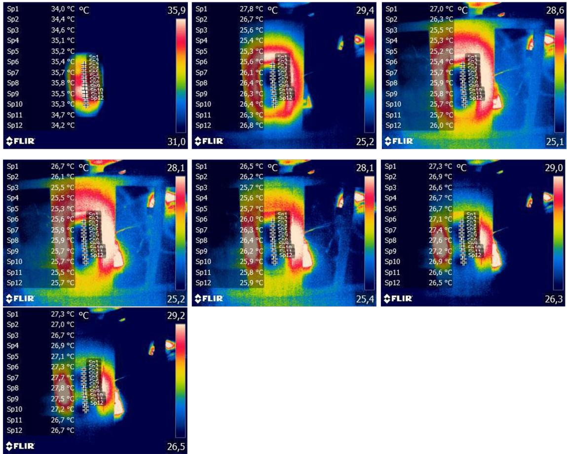
Figure G4: Thermal images of a test of cooling from room temperature. Fluid flow was from sp14 to point sp1 and was  $35 \mu\text{L}/\text{min}$
