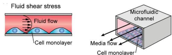
Fig. 1: Schematic drawing of OoC where fluid shear stress can be seen as an active biomechanical stimulus [8]
