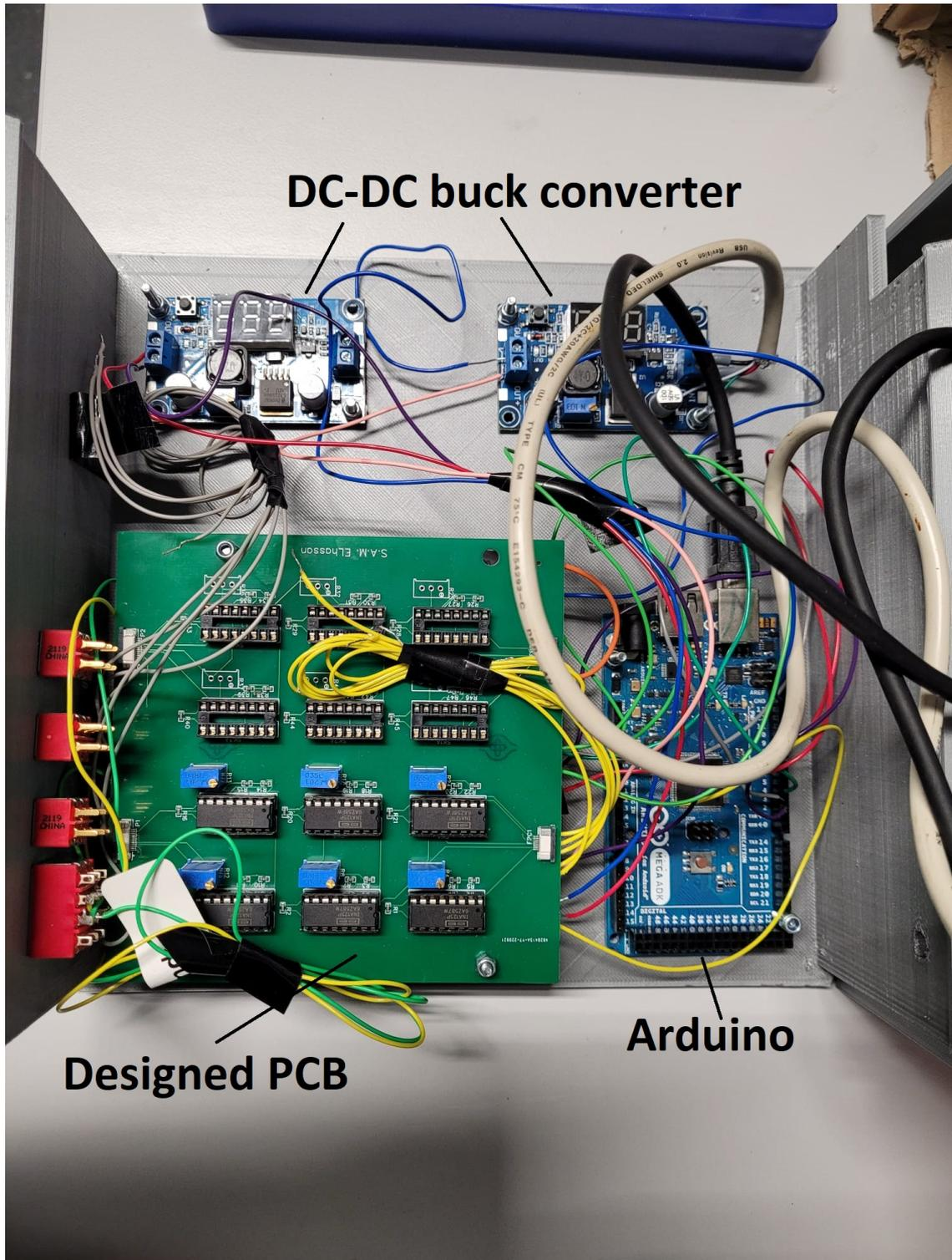
Figure E12: Top view of the electrical components with the PCB for the sensors, the two dc-dc buck converters and the Arduino
