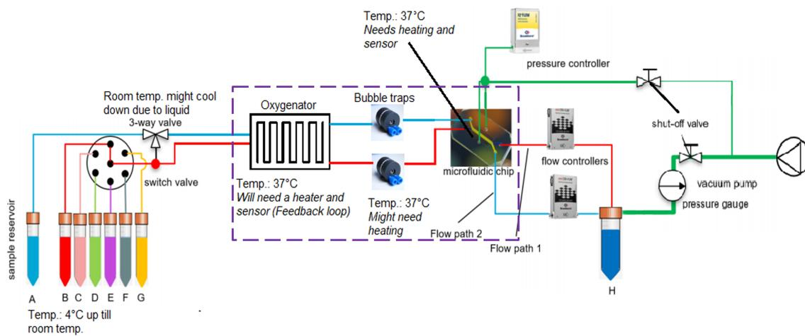
Figure 21: Schematic drawing of the OoC platform. The purple dashed line shows where the temperature control system will be used. This image is an adaptation of the image created by Haoyu Zhu [2]
