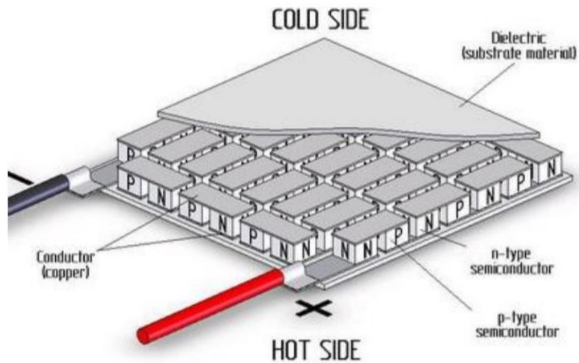
Figure 5: Schematic drawing of a Peltier element [10]
