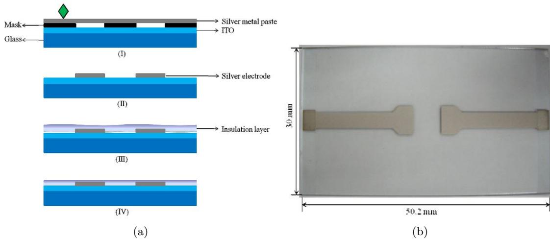
Figure 8: (a) Process steps of the creation of the ITO-glass microheater [13] (b) ITO-glass microheater [13]
