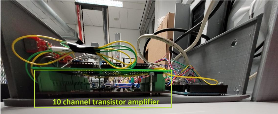
Figure E13: Underneath the PCB for the sensors is the 10 channel transistor amplifier
