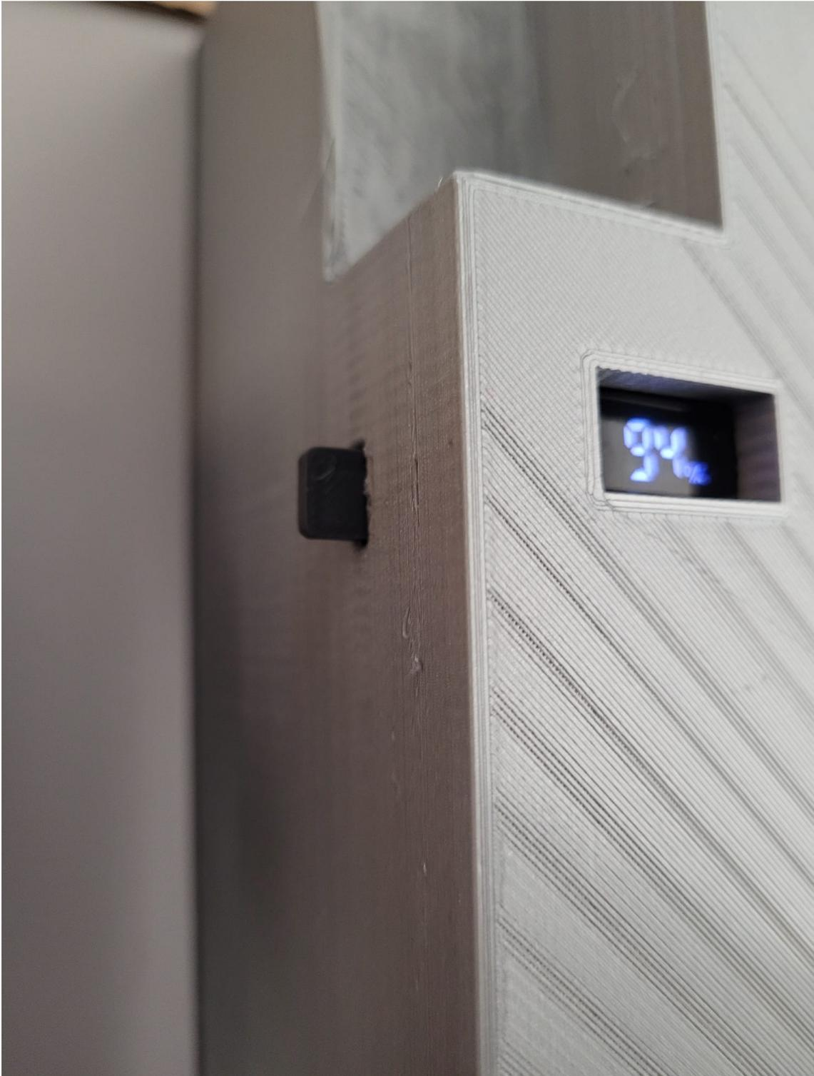
Figure E10: On the side is the on/off button. Pressing once turns the device on. Pressing twice shortly after each other turns the device off
