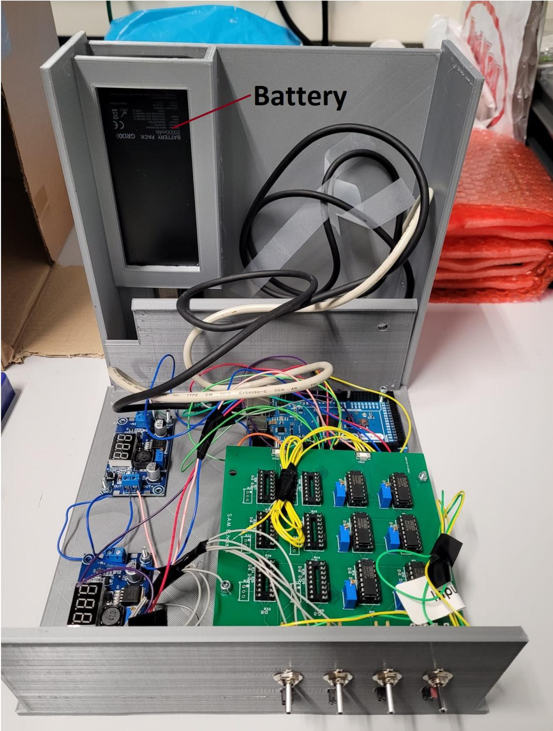
Figure E11: Inside of the box with the electrical components
