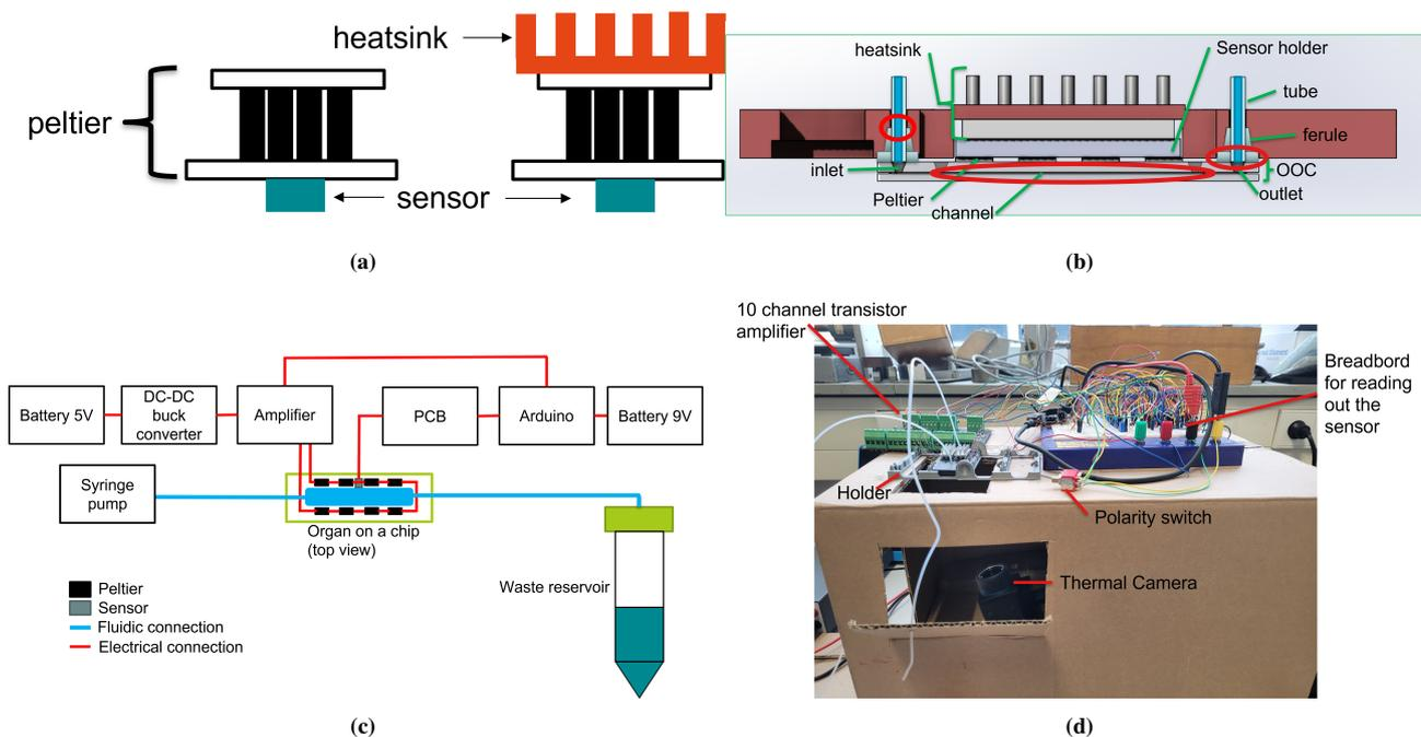
Fig. 5: (a) Schematic drawing of the experimental setup for the understanding of the thermal behaviour of the peltier elements (b) Side view with ferrules and tubings. The red circle shows the areas of possible leakage (c) Schematic drawing of the electronic connection and the fluid connections (d) experimental setup for heating and cooling, the syringe pump and reservoir are not visible but are used during the experiments
