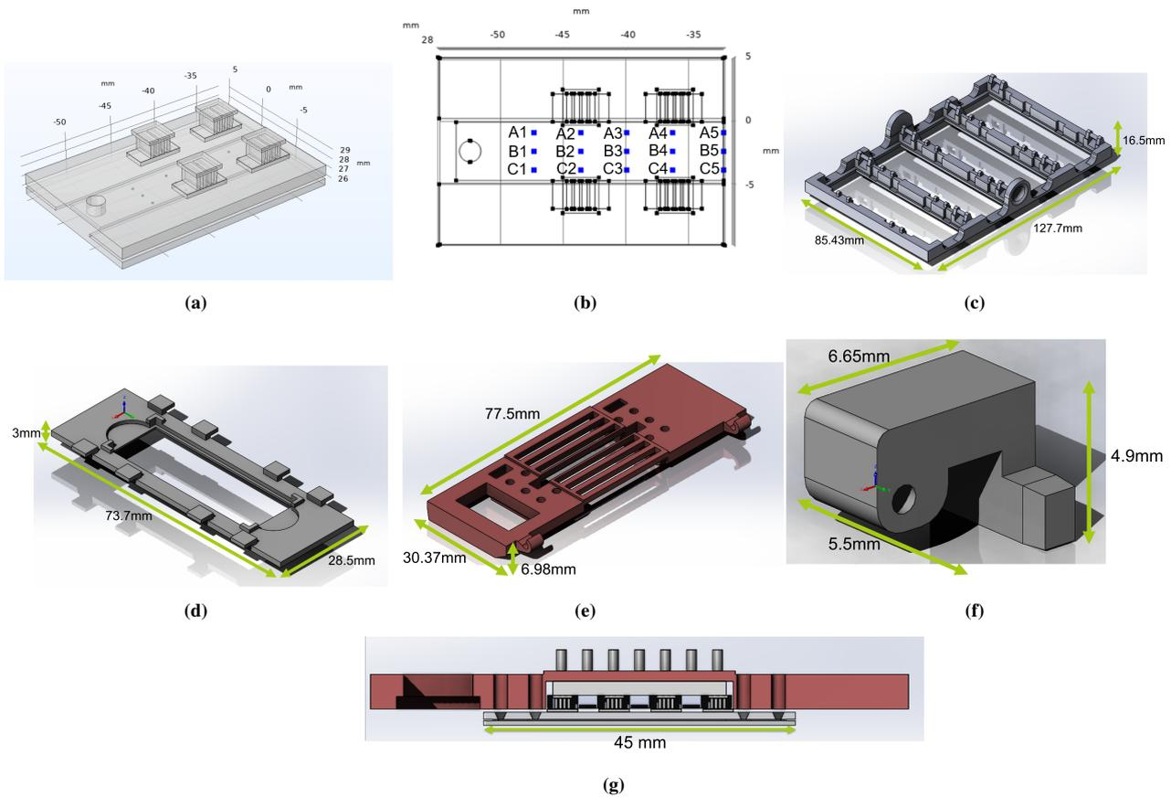
Fig. 3: (a) Numerical model using COMSOL Multiphysics v5.6 (b) Data point position (c) Holder that can hold four chips simultaneously of a maximum size of 75mm x 25mm (glass slide) (d) Chip holder: hold the Micronit chip (e) Lid which will hold the heaters and sensor (f) Lock: which makes sure that the system does not open (g) Side cross-section lid with Micronit chip with a length of 45mm
