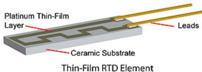
Figure 11: Schematic drawing of an RTD [17]
