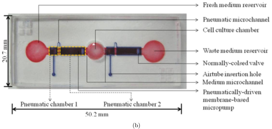
Figure 7: (a) A schematic drawing of the layout designed by Jr-Lung Lin. Where A, B and C are microfabricated PDMS plates. The last rectangular plate is a silver electrode-patterned ITO glass layer [13] (b) Top view of the microfluidic cell culture chip [13]
