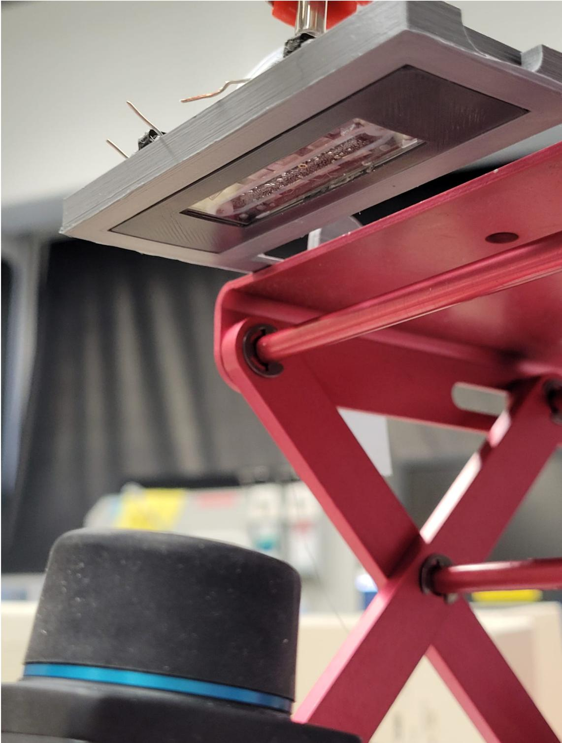
Figure A4: Test setup for Oxygen measurements, view from the bottom of the chip
