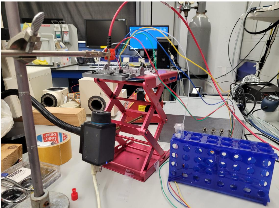
Figure A2: Test setup for Oxygen measurements
