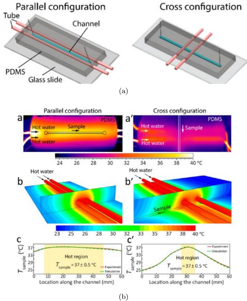
Figure 9: (a) Parallel and cross configuration of the design of Jiu Yang Zhu et al. [14] (b) Result that were obtained by Jiu Yang Zhu et al. [14]
