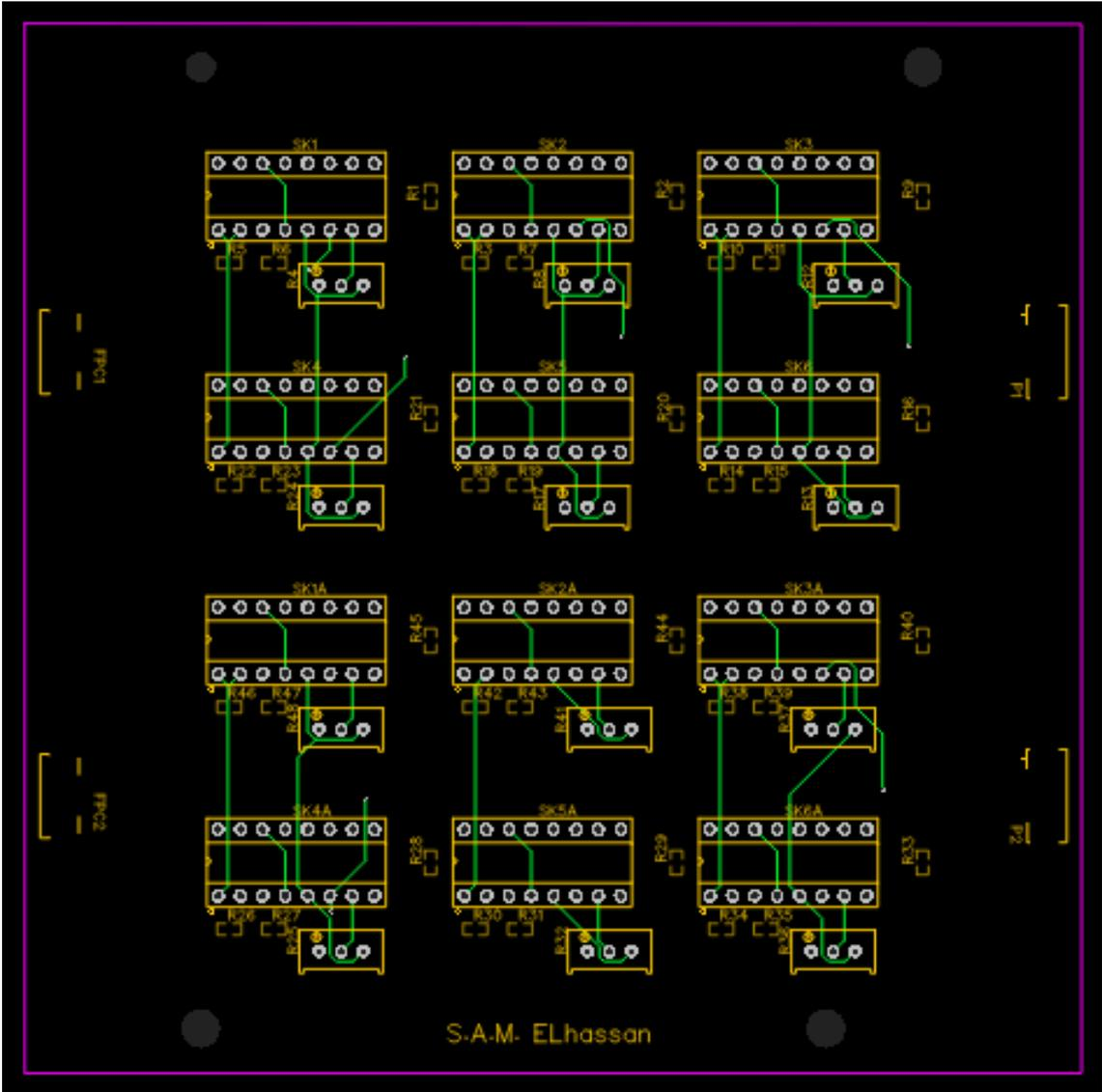
Figure C5: Layout PCB, bottom connections
