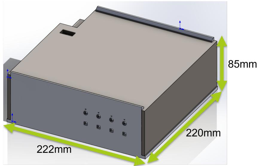
Figure E2: Assembly of the box the circles are for the switches, and the small rectangular holes underneath it are for the cables. The large hole on top is a viewing window for the percentage of the battery
