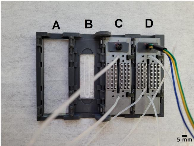
Fig. 4: In area A a glass slide of the dimensions 75 mm x 25 mm is placed. In area B the chip holder and Micronit chip are placed inside of the holder. In area C the lid is placed with the fluidic connections connected to the lid. In area D a cable is connected to the lid for powering the peltier elements and to read out the sensor
