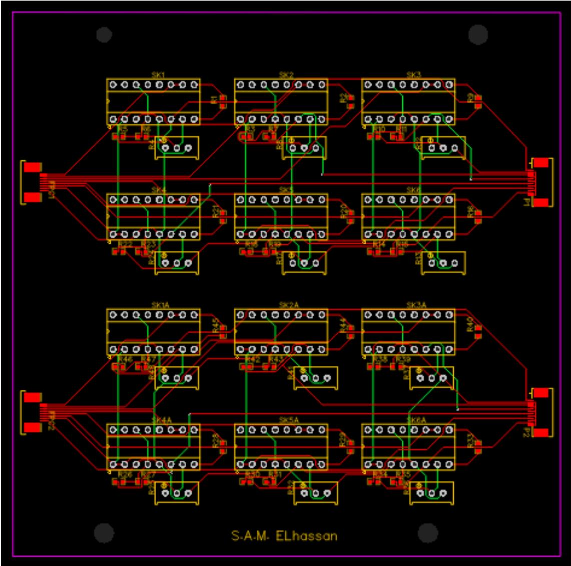
Figure C3: Layout PCB, green are the bottom connection, red the top connections
