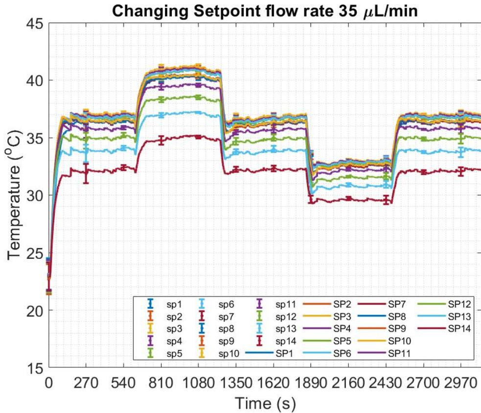
Figure G2: Changing the setpoint from 37  $^{\circ}\text{C}$  to 40  $^{\circ}\text{C}$  back to 37  $^{\circ}\text{C}$  to 34  $^{\circ}\text{C}$  and then back again to 37  $^{\circ}\text{C}$
