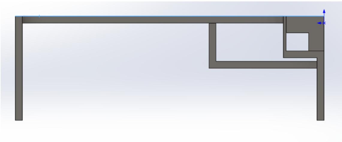
Figure E5: Side view Lid. The rectangular part is to hold the battery
