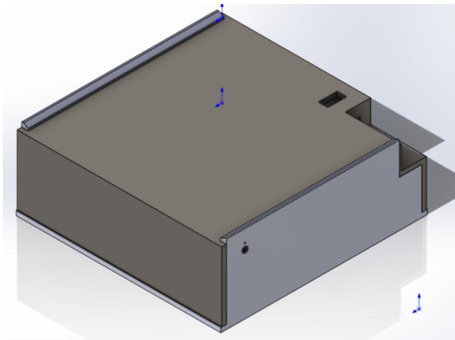
Figure E3: Assembly of the box the circles are for the switches, and the small rectangular holes underneath it are for the cables
