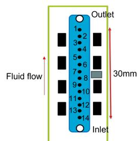
Fig. 6: A schematic drawing of the chip, where the blue rectangle represents the channel, the black rectangles represent the peltier elements and the green rectangle between the peltier elements represents the sensor. Points 1 to 14 are a representation of the locations where the data was collected by the thermal camera. These points were spread over an area a length of 30 mm, which is the length over which the cells will be placed
