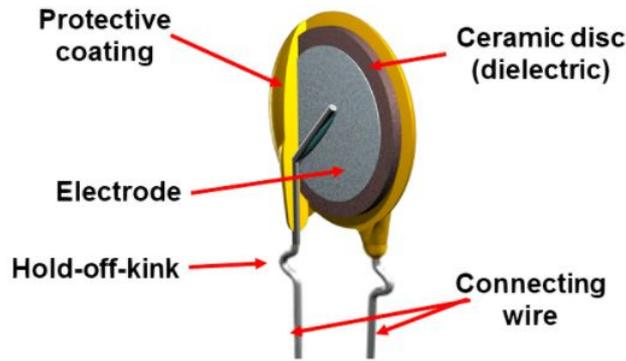
Figure 12: Schematic drawing of a thermistor [18]
