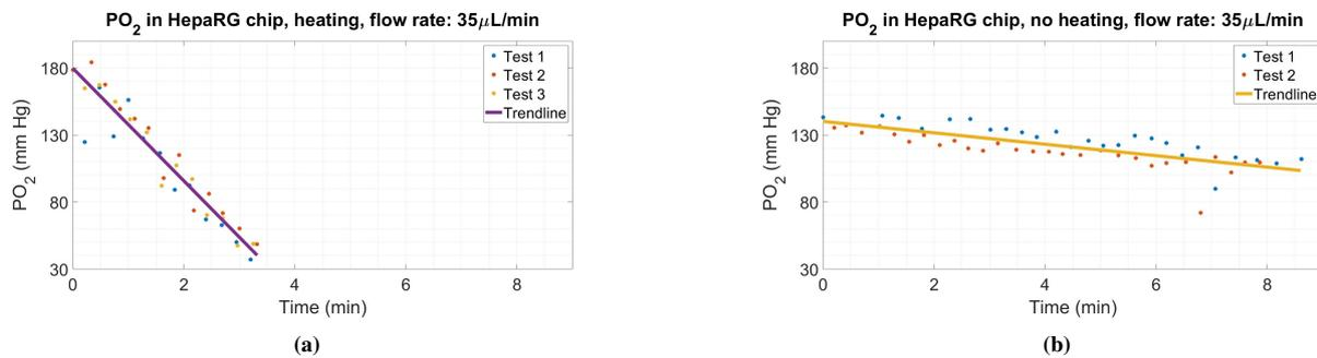
Fig. 10: (a) The  $PO_2$  values of the cells measured when heat is applied. The flow rate of  $35 \mu\text{L}/\text{min}$  was stopped at the start of this graph, thus at  $t=0$  s. (b) The corrected  $PO_2$  values of the cells were measured when no heat was applied. The flow rate of  $35 \mu\text{L}/\text{min}$  was stopped at the start of this graph, thus at  $t=0$  s.
