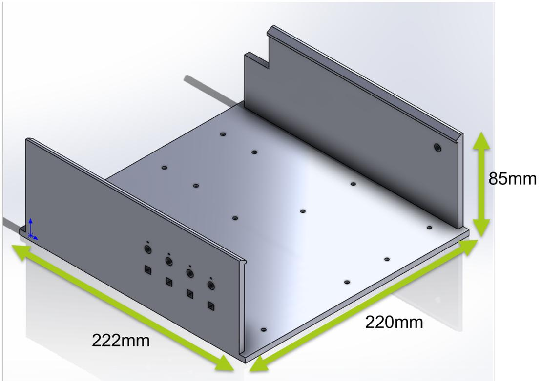
Figure E6: bottom part of the box, holes on the bottom are used to secure the electronic. They can be secured with M3 bolts and screws
