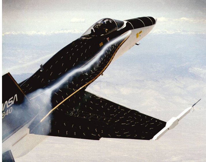
Figure 2.11: F/A-18 smoke and tuft visualisation. NASA Dryden photo EC89-0096-206.
