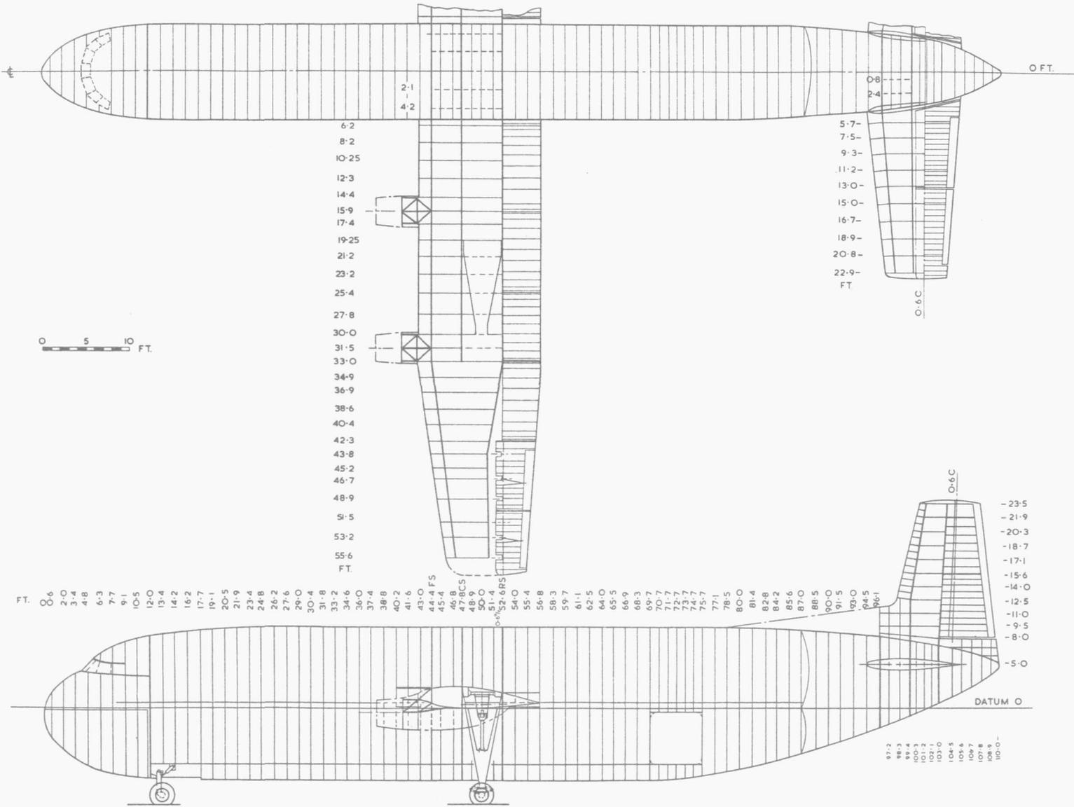
FIG. II STRUCTURAL LAYOUT OF THE GP63
