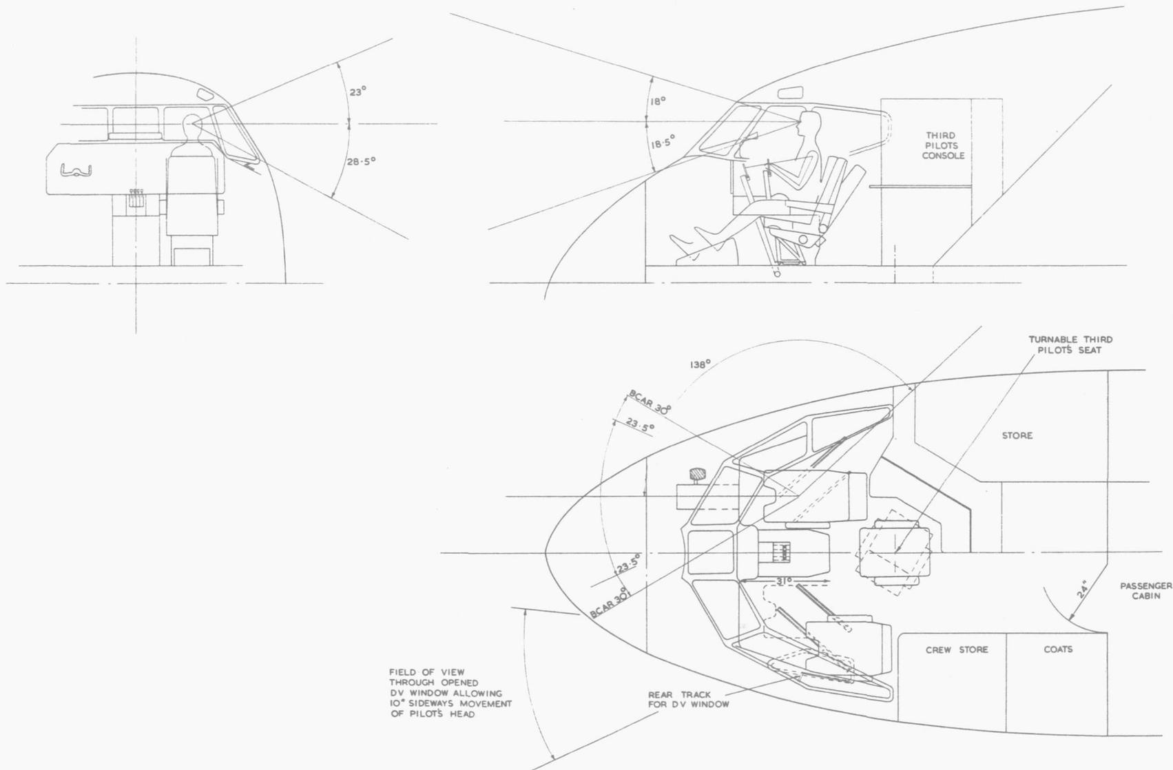
FIG. 16 FLIGHT DECK LAYOUT OF THE GP 65
