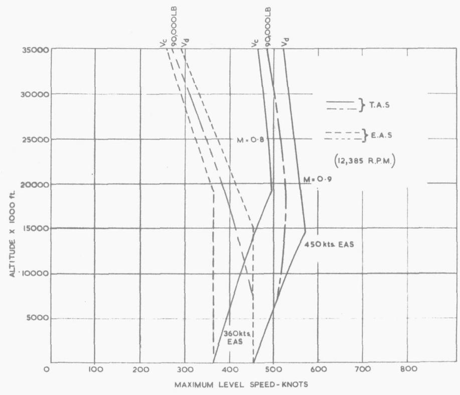
FIG. 10 LEVEL SPEED PERFORMANCE OF THE GP 65
