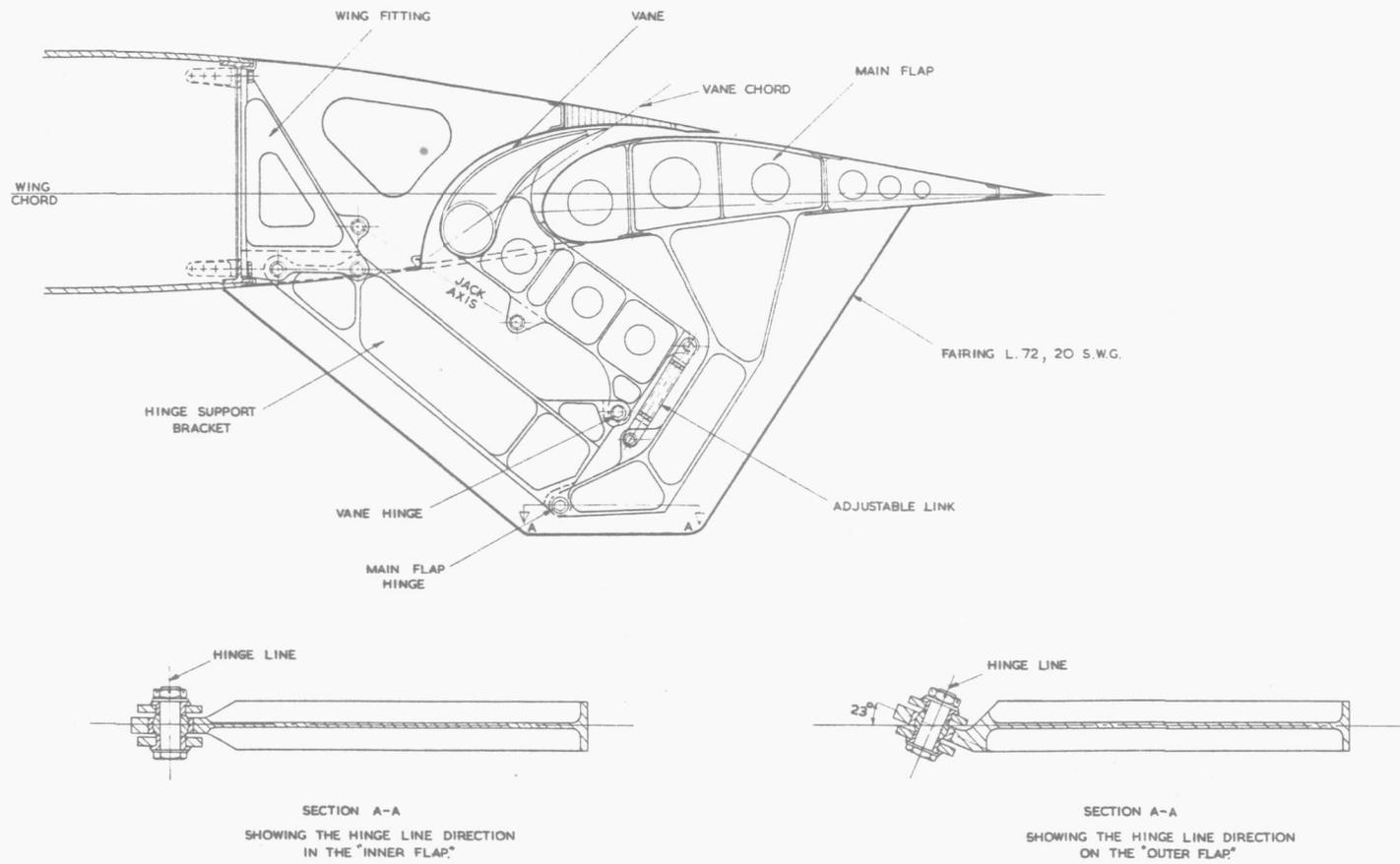
FIG. 15 FLAP MECHANISM OF THE GP 65
