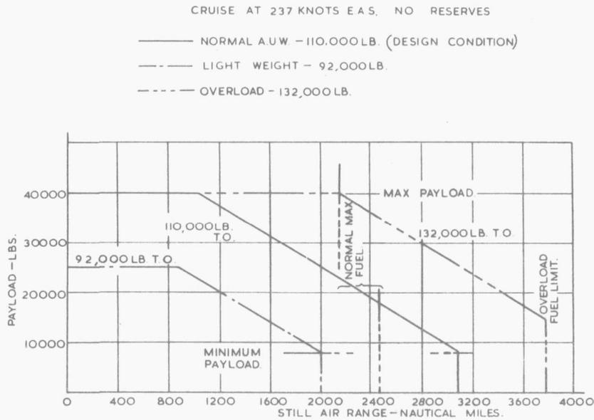
FIG. 7 PAYLOAD - RANGE PERFORMANCE OF THE GP 63
