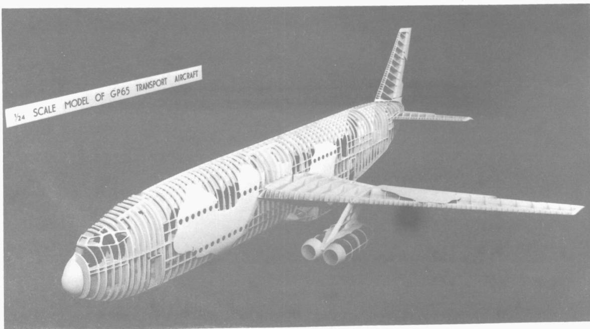
FIG. 20            STRUCTURAL MODEL OF THE GP65
