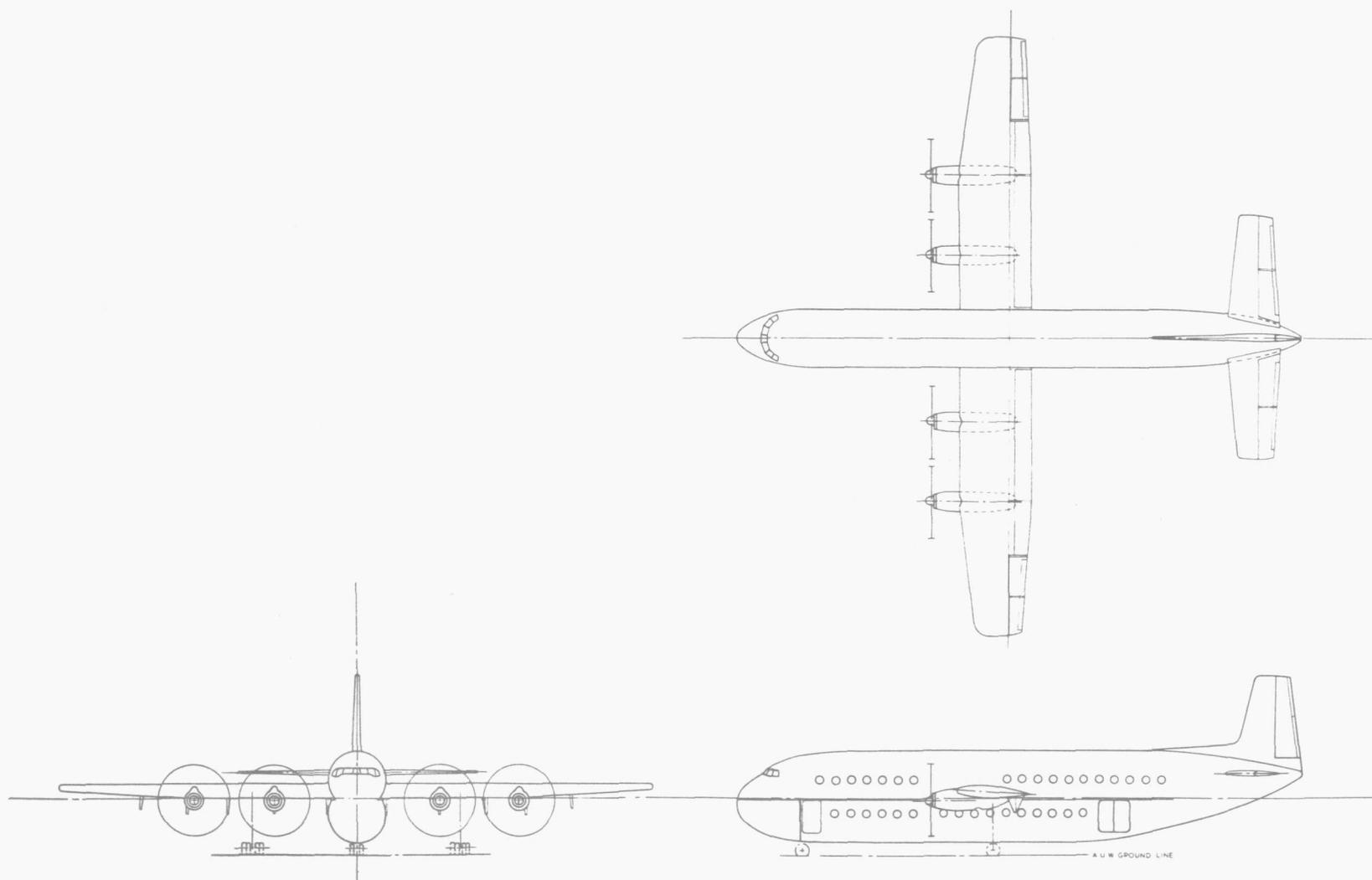
FIG. I GENERAL ARRANGEMENT OF THE GP 63
