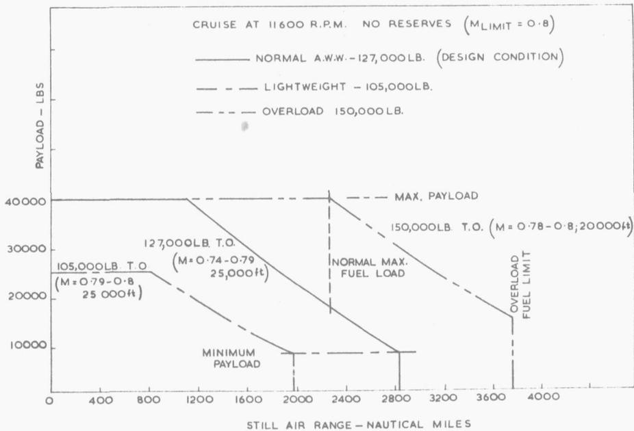
FIG. 8 PAYLOAD - RANGE PERFORMANCE OF THE GP 65
