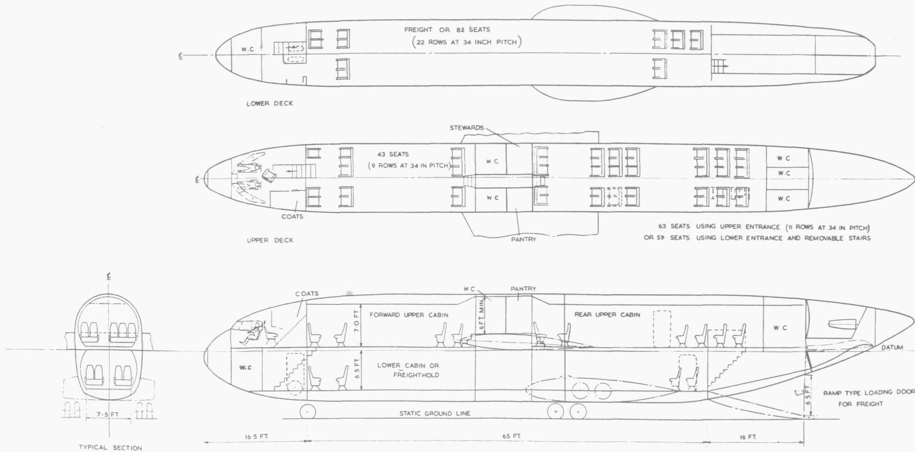
FIG. 6 FUSELAGE LAYOUT OF THE GP 65
