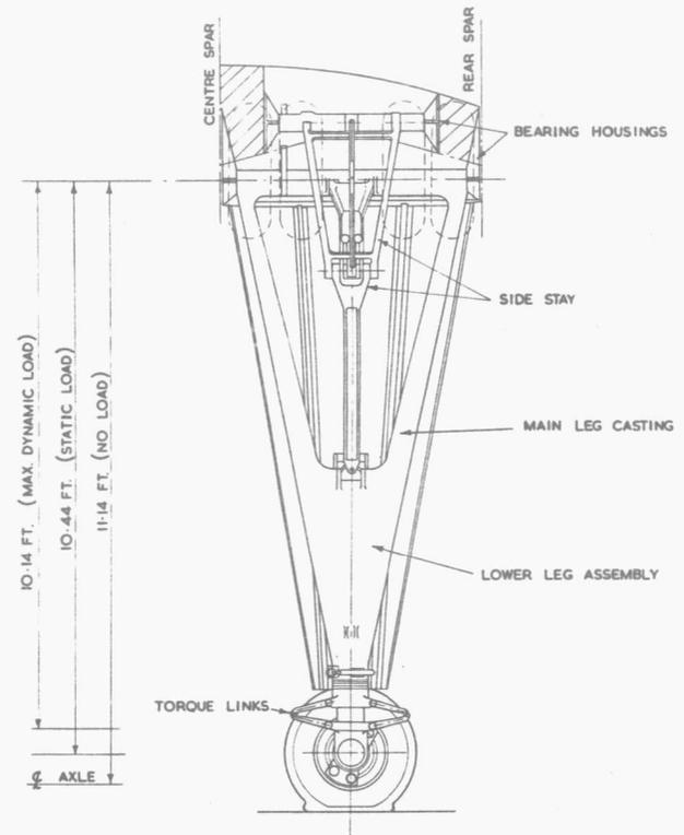
FIG. 14 LAYOUT OF THE UNDERCARRIAGE OF THE GP 63
