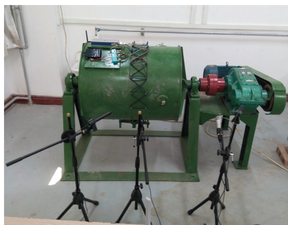
Fig. 5. Ball mill equipment used in the experiments.
