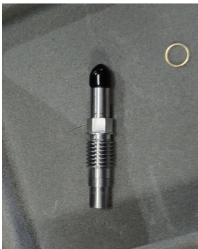
Figure D.1: PCB 112A22. The sensing membrane is located at the bottom and the electrical connector at the top.
