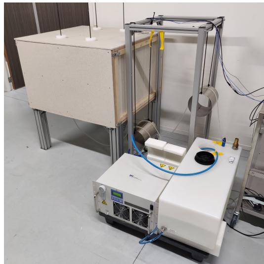
Figure 4.5: Picture of the setup with the lid of the acoustic enclosure closed
