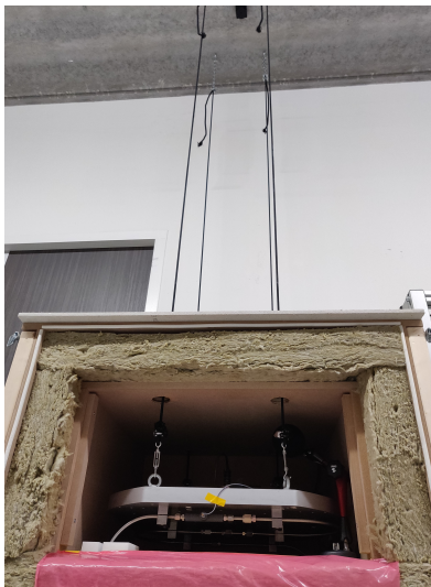
Figure 4.4: Picture of the setup with the lid of the acoustic enclosure open
