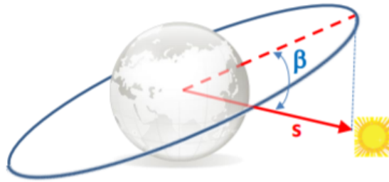
Figure 5.14: Visualisation of the beta angle \beta , from [37]
