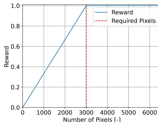
Figure 5.5: Reward system for the payload subsystem
