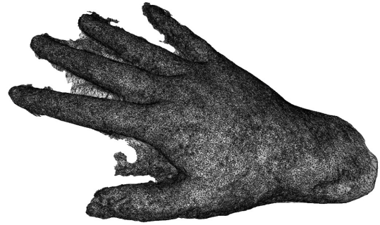
Figure 3.2: 3D model of part of the hand using the time-of-flight principle.
