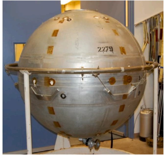
Fig. 3. Aluminium receiver tank [22].
