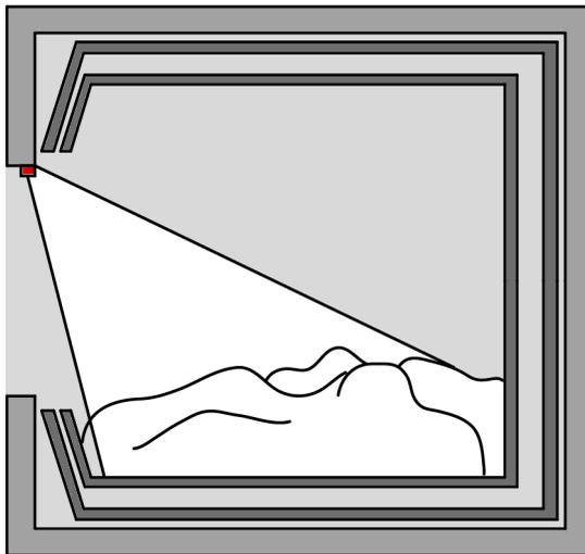
Figure 65: LED shining on the laundry in the wash drum
