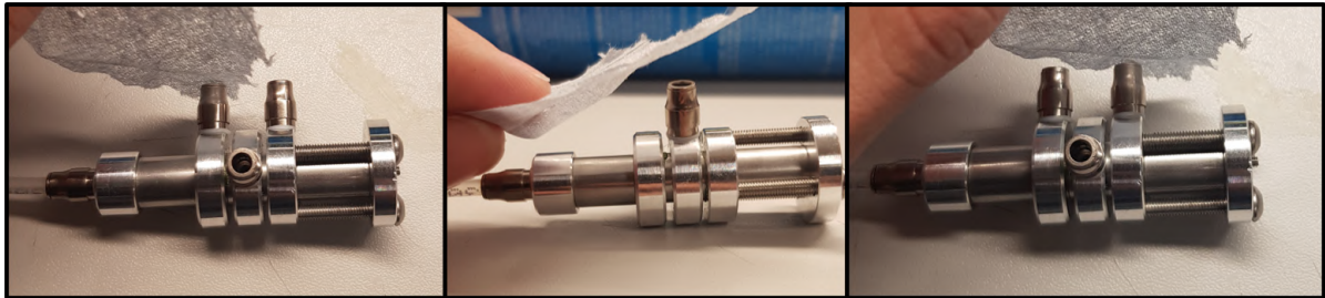
Figure 6.5: Response of the pressure regulator to a moderate pneumatic inlet flow. Here it can be seen that the CO 2 flows from the inlet to the second outlet, i.e. the outlet leading to the locking mechanism.
