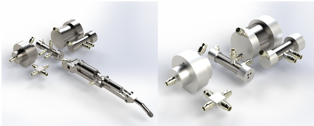
Figure 5.1: Overview of the design of the first two versions of the prototype for the pneumatic hand prosthesis. Left: first version of the prototype, consisting of the transmission cylinders, pressure regulator, a finger and tube couplings. Right: second version of the prototype, consisting of the transmission cylinders, pressure regulator and tube couplings.
