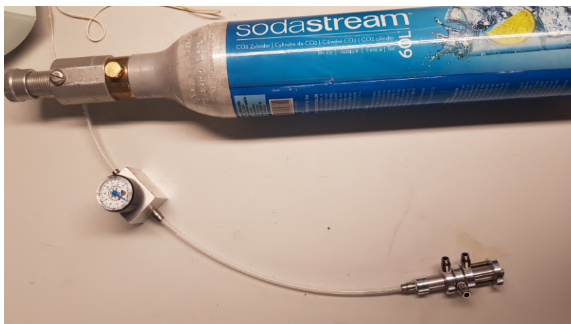
Figure 6.3: Setup used for pneumatic testing, in this case the pressure regulator is attached. A CO 2 supply consisting of a SodaStream canister with a flow regulating valve, is connected to a manometer, which in turn is connected to the pneumatic inlet of the component that will be pressurized.
