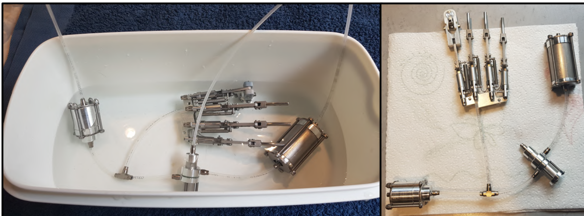
Figure 6.14: Left: hydraulic side of the prototype submerged in water, in order to fill it with water and seal it without air entering the system. Right: The filled and sealed off hydraulic side of the prototype.
