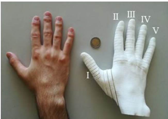
Fig. 25. 3D printed soft prosthetic hand of Almeida et al. [17] based on the 3D scans of the adjacent human hand. The segmentation of the fingers allows them to bend similarly to a human hand.
