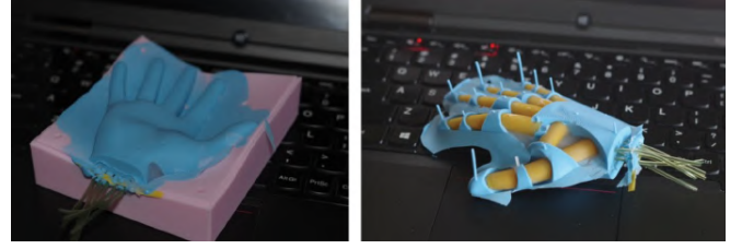
Fig. 6. Molding of the exoskeleton of a prosthetic hand (blue) around the soft pneumatic actuators (yellow) in [25], using a 3D printed mold.
