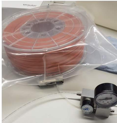
Figure 6.16: Picture of the loaded test where a heavy object, in this case a big roll of 3D printer filament is placed on top of the finger.
