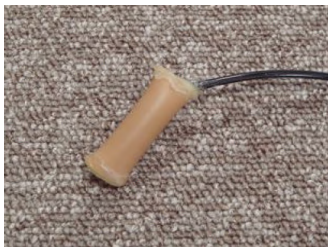
Fig. 14. Balloon sensor developed by Kadota et al. [45]. It consists of a rubber tube, closed on one end and connected to a differential pressure sensor through a tube on the other end.
