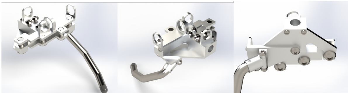
Figure 4.14: Three different views of the palm base, including the thumb, of the design of the hand prosthesis. Each of the four fingers is attached with one of the four M6 screws at the front of the palm. On top of the palm, the connectors for the transmission cylinders and pressure regulator are visible.
