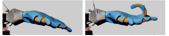
Fig. 7. Pressurization of a single soft pneumatic actuator of the soft prosthetic hand of Fras and Althoefer [25], resulting in the bending of the pressurized finger.
