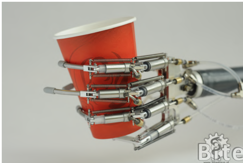
Figure 1.3: Image of the Delft Cylinder Hand [9] without its cosmetic cover and holding a coffee cup.
