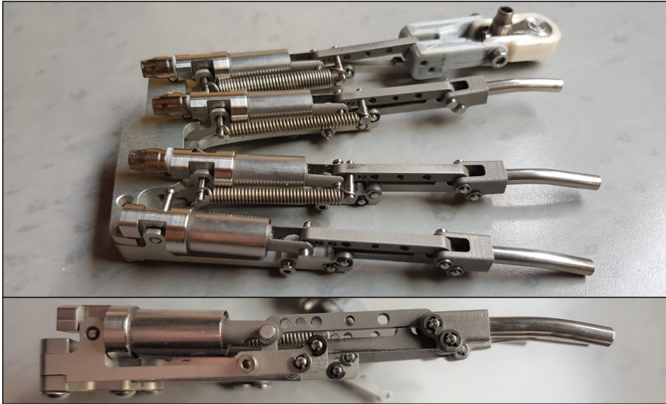
Figure 6.2: The hydraulic hand prosthesis of which one finger was used for testing the prototype. Top picture: overview of the hand that was used, consisting of four fingers. Bottom picture: side view of the hand, showing the construction of a finger.
