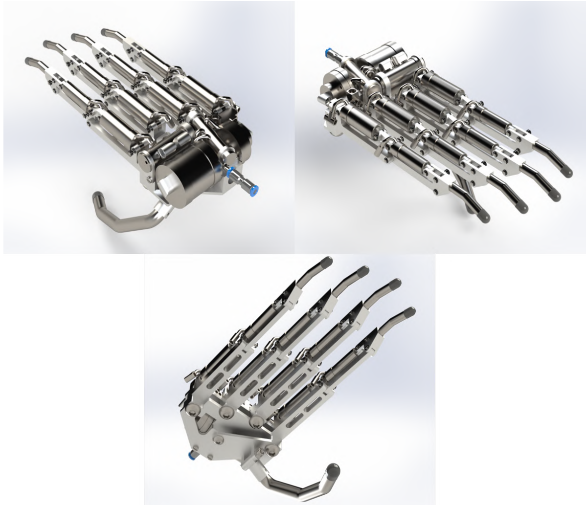
Figure 4.15: Three different views of the complete design of the pneumatically powered hand prosthesis, excluding the tension springs on the fingers and the pneumatic tubing.
