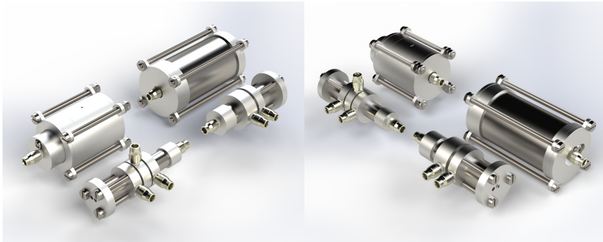
Figure 5.11: Two different views of the fourth design for a prototype for the pneumatic hand prosthesis, consisting of the transmission cylinders and pressure regulator.
