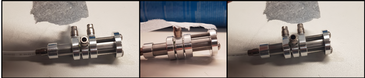
Figure 6.4: Response of the pressure regulator to a low pneumatic inlet flow. Here it can be seen that the CO 2 flows from the inlet to the first outlet, i.e. the outlet leading to the high stroke cylinder.
