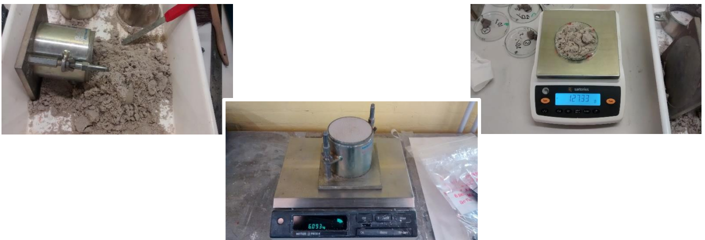
FIGURE 4 – EMPTYING OF MOLD, WEIGHING THE FILLED MOLD, WEIGHING A SAMPLE FOR WATER CONTENT (LEFT TO RIGHT)
