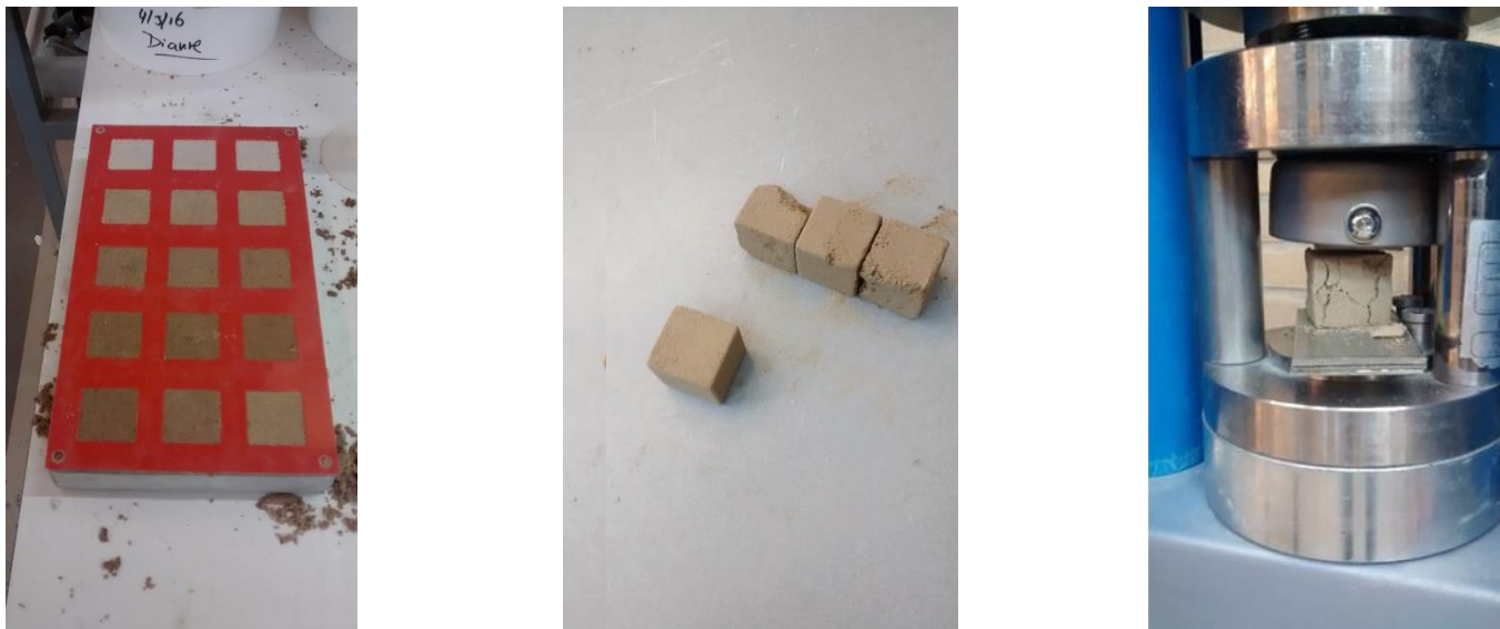
FIGURE 8 – MIXES FILLED IN MOLD, DAMAGED DRIED CUBES, CUBE IN UCS TEST MACHINE (LEFT TO RIGHT)
