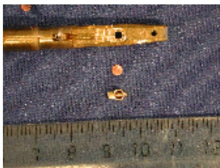
Figure 6-15: The gas cell together with the typical TEM specimen and specimen holder.
