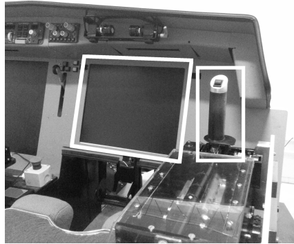
Figure 4.2: The apparatus used in the JND experiment. The side-stick manipulator and the LCD screen are marked by white rectangles. The manipulator could be deflected laterally (left/right) like a joystick. The LCD screen only displays the visual presentation of the tracking task.
