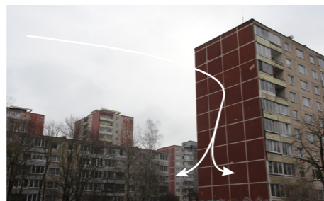
Figure 176. Tall building downdraft
