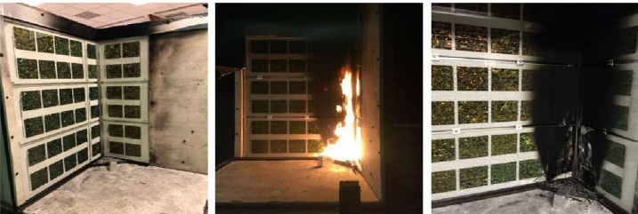
Figure 1: SBI-test with PIZ BIPV cladding system. Source: IEA PVPS Task 15 (2023)
