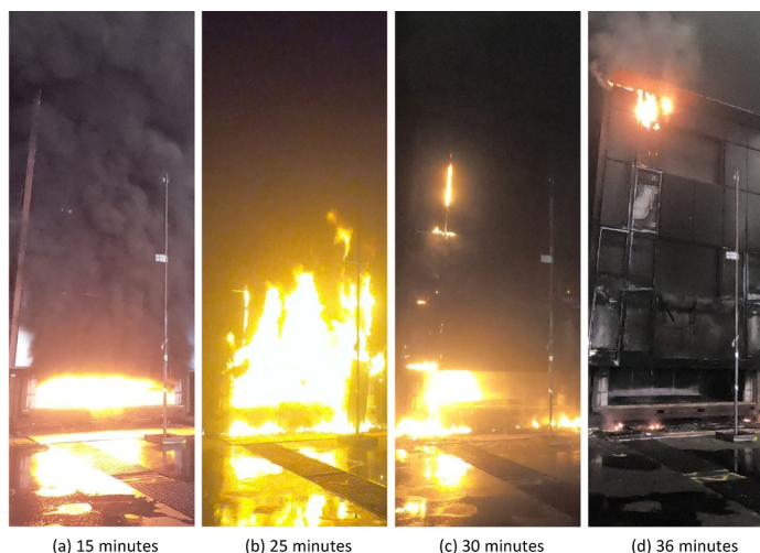
Figure 61: Large scale test BIPV façade. Impact falling BIPV modules. Source: Stølen et al. (2024)
