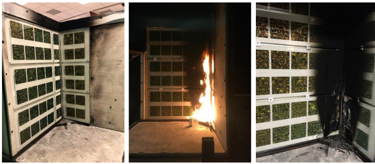
Figure 40: SBI-test with PIZ BIPV cladding system. Source: IEA PVPS Task 15 (2023)
