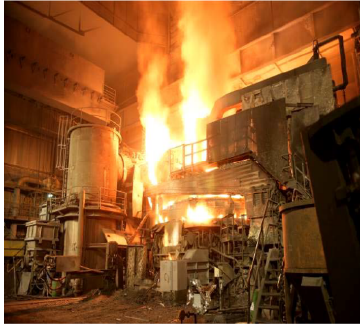
Figure 2-3: Electric arc furnace ArcelorMittal Hamburg (By Author)
