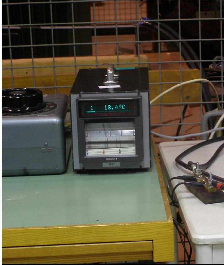
Figure 7.4 the recorder and the variac (adjustable current source) used in the laboratory
