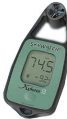
Figure 7.3 the Fluke Ti50 infrared camera (left) used for the temperature measurements and the Skywatch Xplorer2 (right) wind meter to record the wind speed
