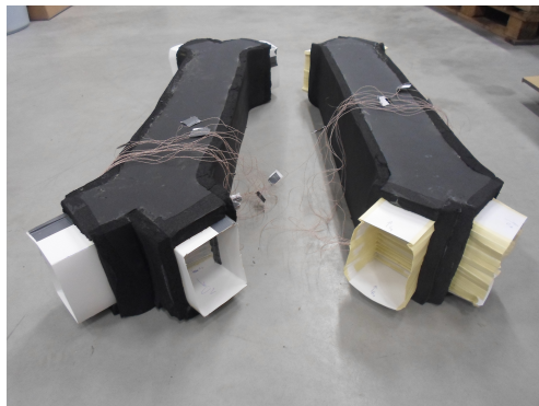
Figure E-1: Two heat exchangers, insulated and prepared for testing
