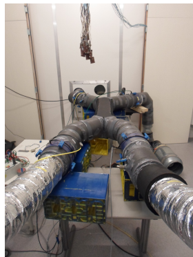
Figure E-2: Heat exchanger test in climate chamber
