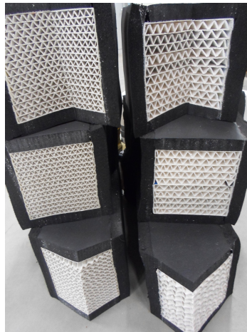
Figure E-4: After testing. Different channel size of both heat exchangers
