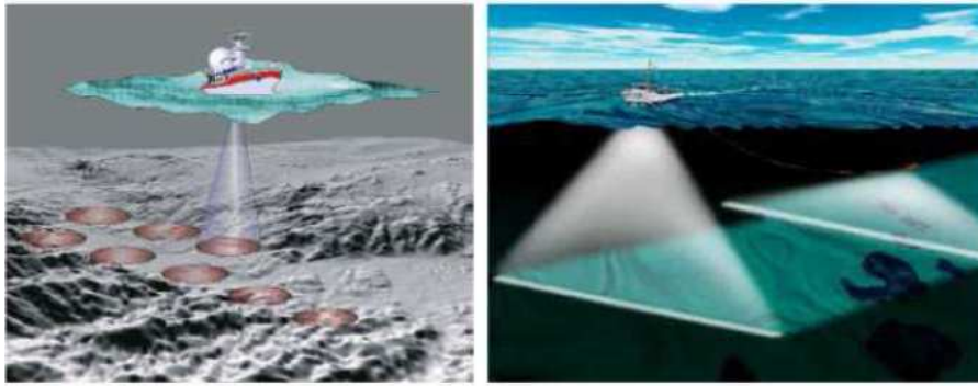
Figure 2.2: Echo sounding systems. On the left: Single-beam echo sounding. On the right: Multi-beam echo sounding and a side-scan sonar mounted on a towfish, behind the vessel. Source: [16].
