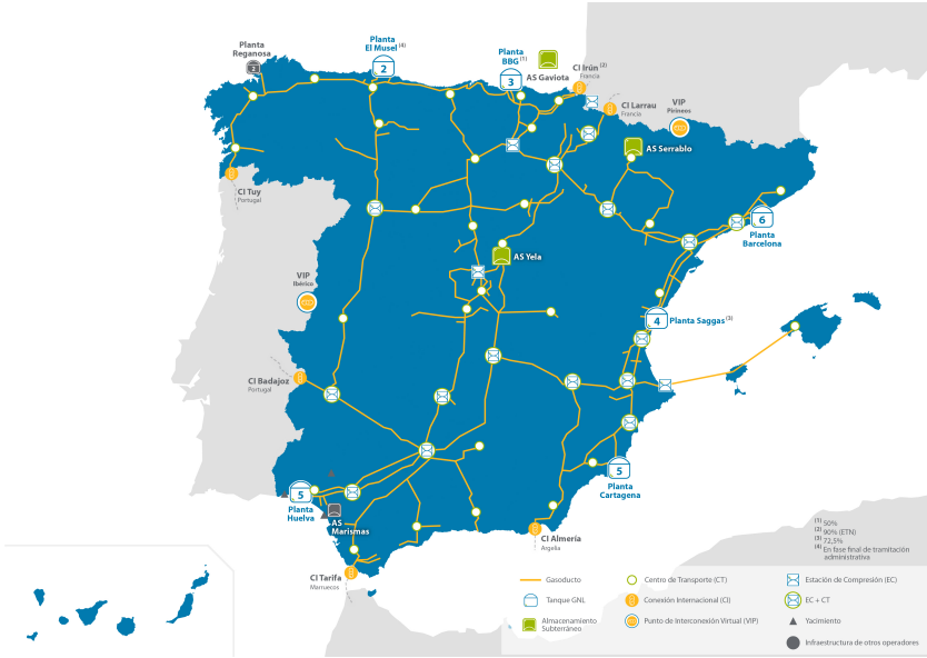
Figure A.4: Map of the 2022 Spanish gas network according to Enagas [34]
