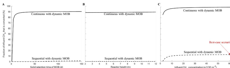
= 150 d) and tall reactor ( $H = 12$  m) were used to obtain a best-case scenario at the highest influent concentration, while all other parameters were set at their reference value.
