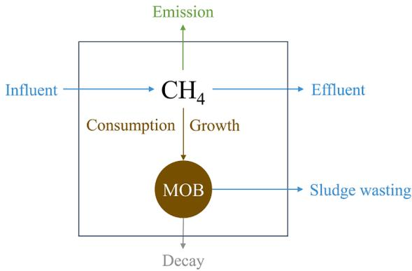
Fig. 2. Sinks and sources of methane (CH<sub>4</sub>) and methane oxidizing bacteria (MOB) considered in the simple model.
