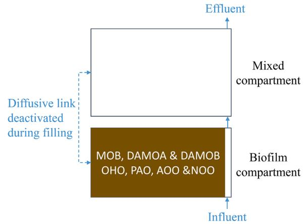
Fig. 4. Representation of the multi-species and multi-substrate biofilm kinetics, anoxic methane consumers and high substrate concentrations in the settled sludge bed during upward plug flow feeding in the rigorous model.
