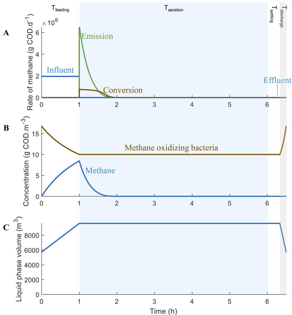
Fig. 6. Cyclic changes in a sequentially operated reactor with a fixed amount of biomass ( $X_{MOB} = 10 \text{ g COD.m}^{-3}$  during the aeration phase) simulated with the simple model. (A) Rate of methane input, emission, conversion and output. (B) Concentration of methane and methane oxidizing bacteria. (C) Mixed liquor volume in the reactor. All parameters were set at their reference value (Table 1).
