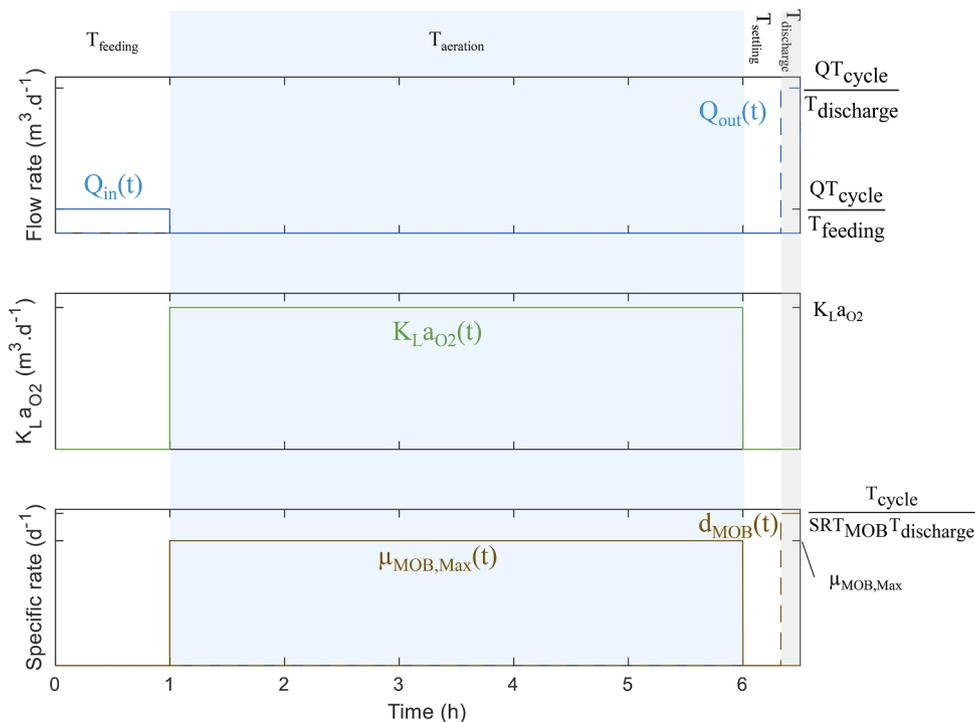
Fig. 3. Periodic variation of the parameters  $Q_{\text{in}}^L$ ,  $Q_{\text{out}}^L$ ,  $K_{\text{L}a_{\text{O}_2}}$ ,  $\mu_{\text{MOB,Max}}$  and  $d_{\text{MOB}}$  during one cycle of a sequentially operated reactor.
