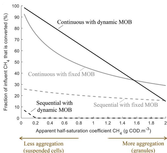
Fig. 8. Effect of the apparent half-saturation coefficient of methane  $K_{\text{CH}_4, \text{MOB}}$  on the methane conversion efficiency simulated with the simple model. The range of  $K_{\text{CH}_4, \text{MOB}}$  values reflects the anticipated range from suspended cells over flocs to granules (Arcangeli and Arvin, 1999). All other parameters were set at their reference value (Table 1).
