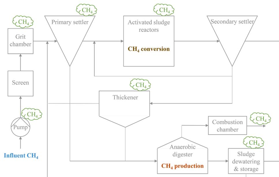
Fig. 1. Typical hot-spots of methane input, production, emission and conversion (biological oxidation) in a wastewater treatment plant, indicated with green clouds.
