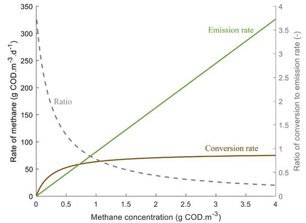
Fig. 7. Emission and conversion rate and their respective ratio as a function of the dissolved methane concentration for an apparent half-saturation coefficient  $K_{CH_4,MOB} = 0.26 \text{ g COD.m}^{-3}$ , concentration of methane oxidizing bacteria  $X_{MOB} = 10 \text{ g COD.m}^{-3}$  and volumetric overall transfer coefficient of oxygen  $K_{l,aO_2} = 100 \text{ d}^{-1}$ , simulated with the simple model.
