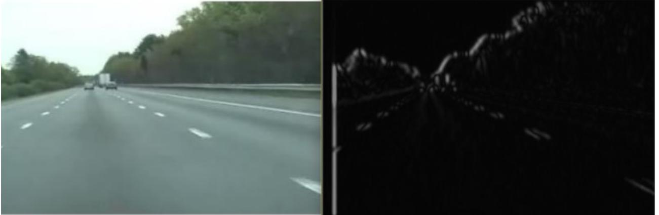
**Figure 2-7:** Before(left) and after(right) applying canny edge detection
