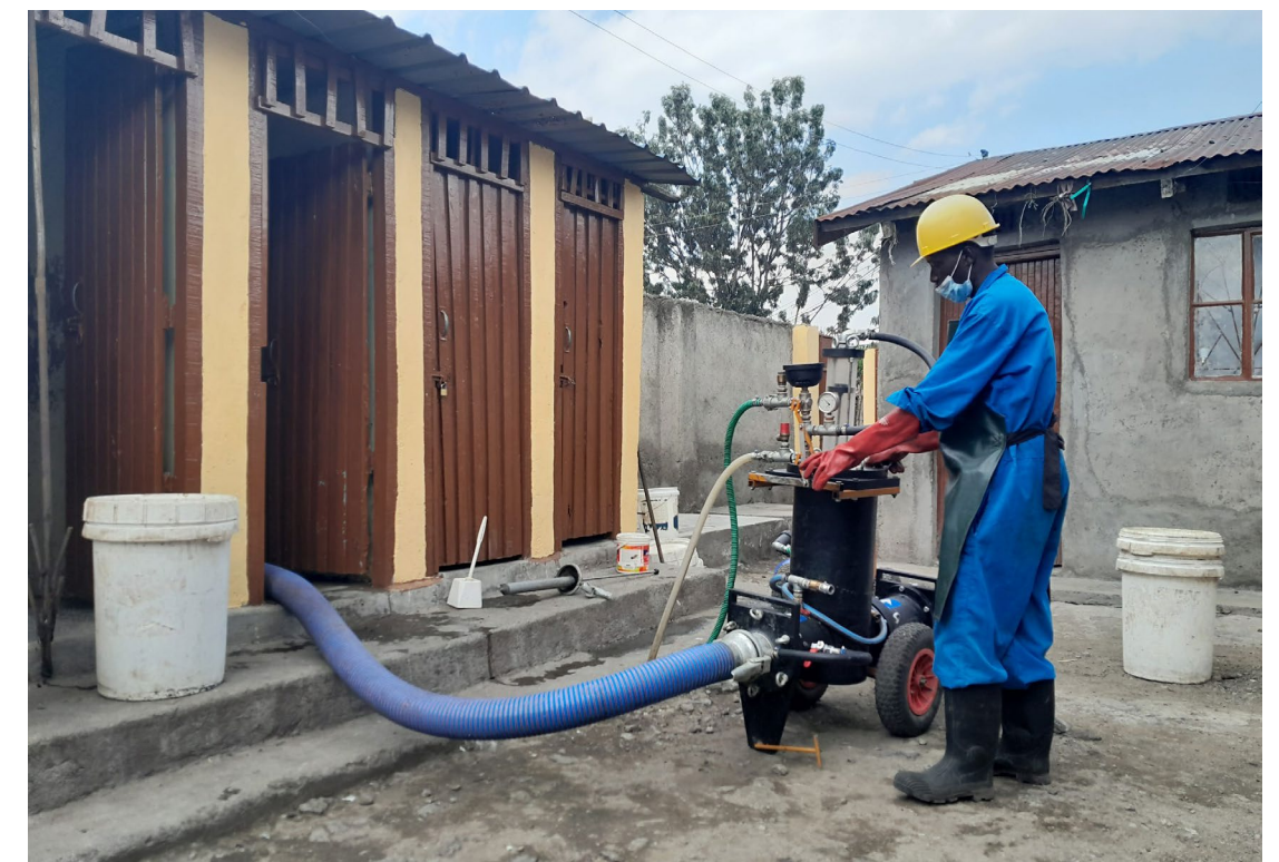
Fig. 4.8 | The Pupu Pump being used to empty a latrine
