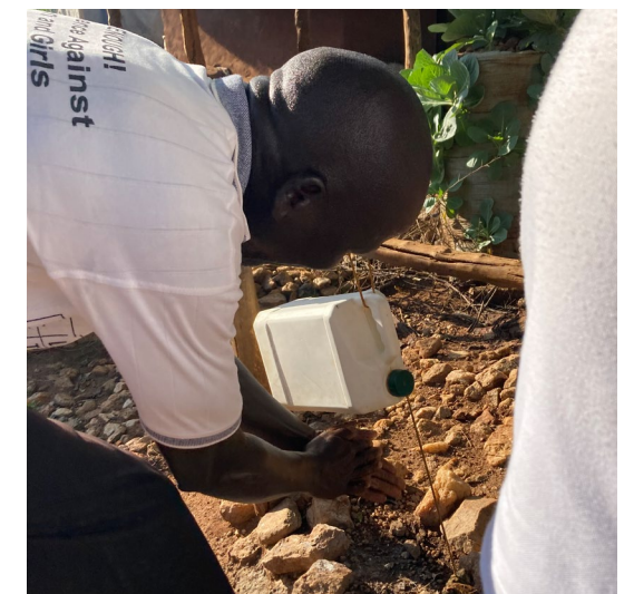
Fig. 2.21 | Handsfree hand washing facility using sticks, rope and a jerrycan
