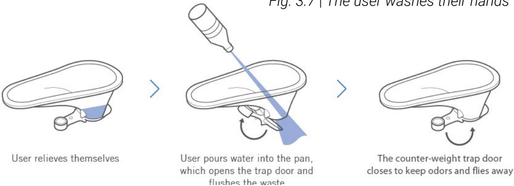
Fig. 3.8 | Flushing the Sato toilets (SaTo Pans – WaterSchool, n.d.)
