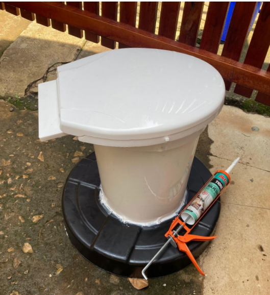
Fig. 3.20 | The first prototype toilet bowl
