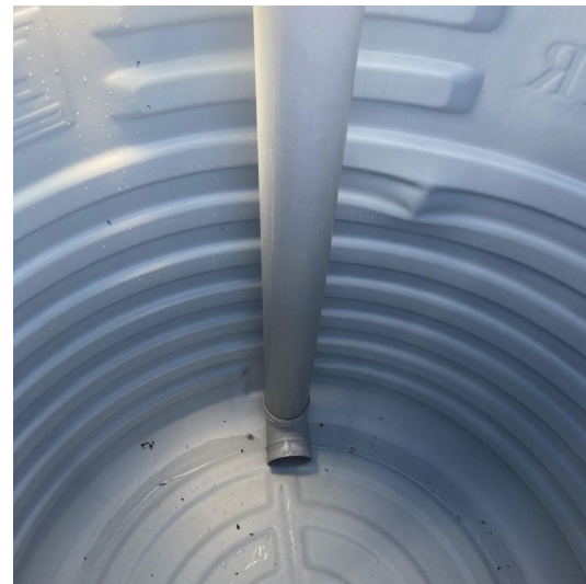
Fig. 3.16 | Prototype 1's internal pipe for sludge emptying
