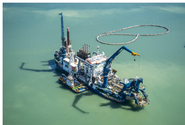
Fig. 1. Cutter Suction Dredger 'Athena' owned by van Oord.
