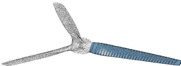
Figure 3. 3D scan of the propeller (black dots) and blade reconstruction in CATIA™.
