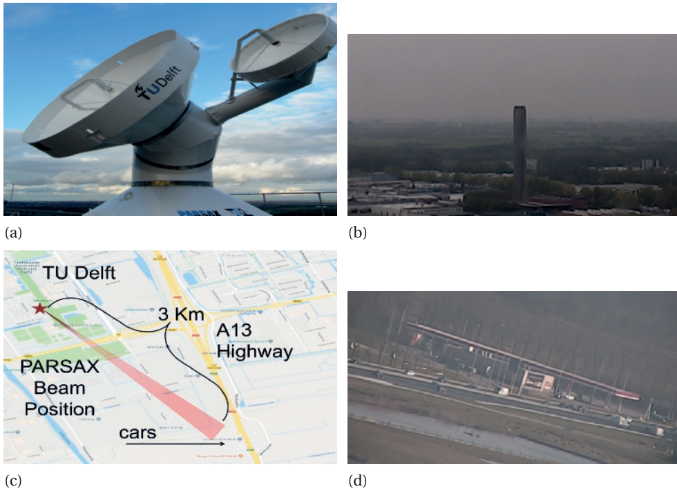
Figure 2.8: Experimental setup. (a) The PARSAX radar (b) Industrial chimney as a stable-target in experiment 1 (c) location of highway in relation to PARSAX for experiment 2 (d) Photo of the illuminated highway area for experiment 2.
