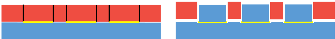
Figure 4.2: Production steps using laser cutter, first glue two plates partially together at the yellow locations, then use the laser cutter to make cuts over the black lines. Then the top and bottom plate can be separated.
