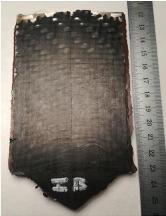
Fig. 7. Macroscopic view of the G-Weave plate impregnated at 240 °C without spacer.
