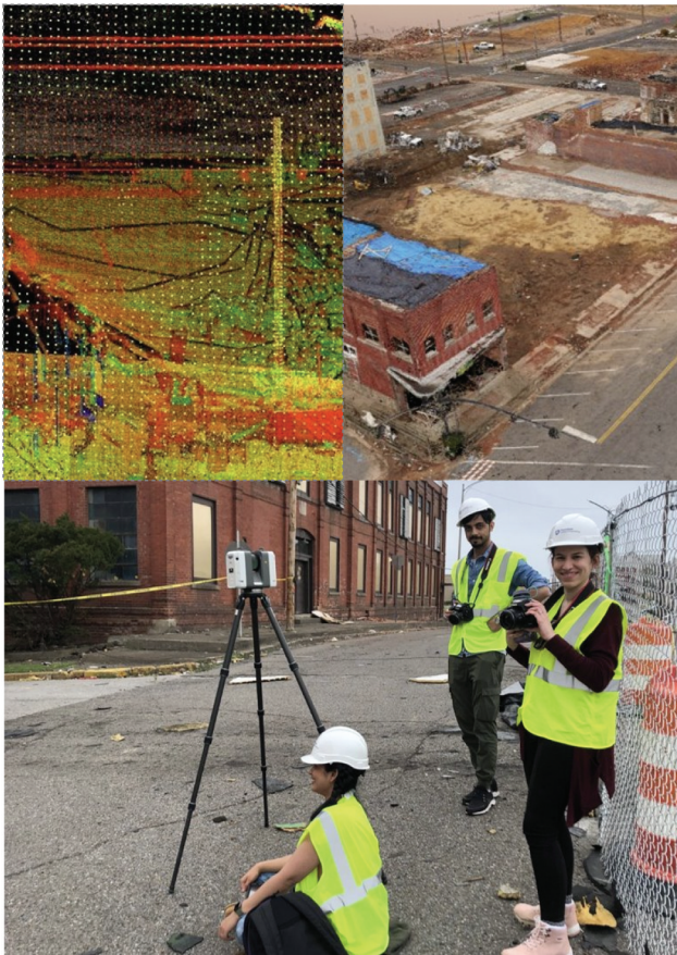
Figure 2. High-precision digital documentation using a terrestrial laser scanner at a heritage site after a tornado. The top left panel is a close up of the 3D model; the top right panel is a top down view of the 3D model; the bottom panel is a picture of student researchers capturing the point cloud after the tornado.
